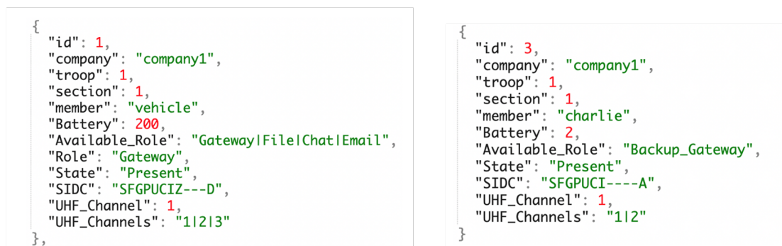
Figure 9.12: JSON representation of two radios each with different configurations.
