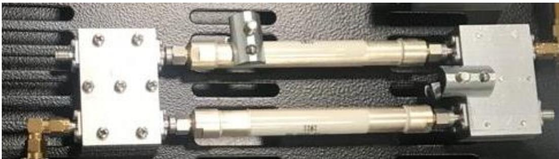
Figure 3-4: Diplexer, including low pass filters and hybrid couplers
