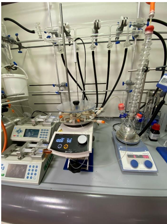
Pictures of setup – Large scale setup with top view of fReactor in action
