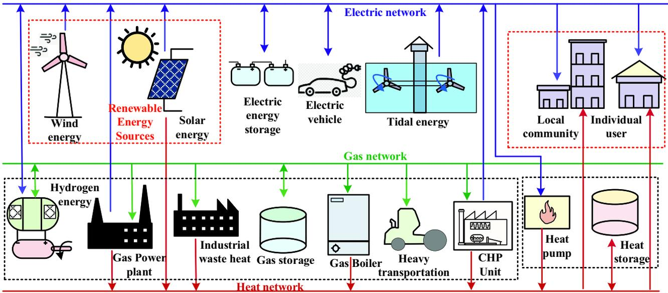
FIGURE 1 Schematic of interaction between electric network, heat network and gas network
