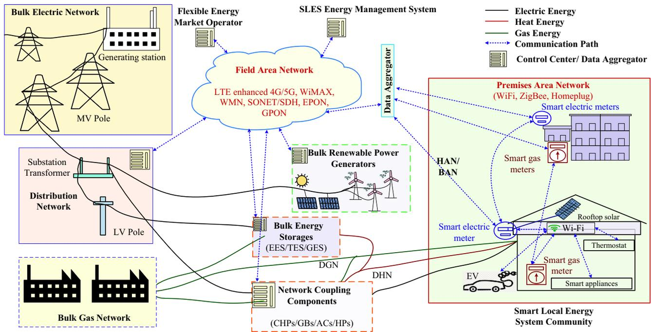
FIGURE 3 An example of communications infrastructure in smart local energy systems (SLES)
