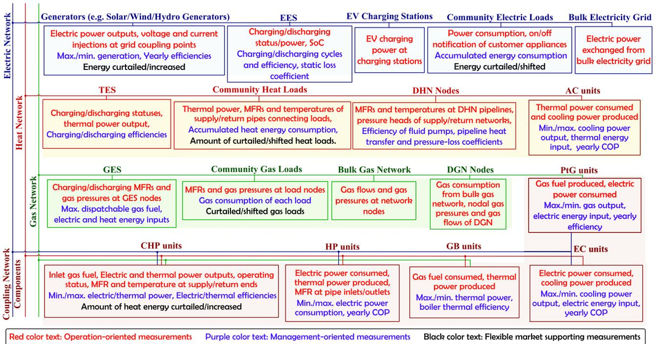
FIGURE 2 Key measurements associated with multi-carrier local energy networks
