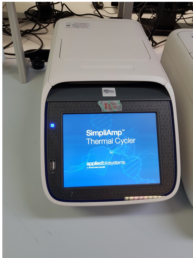
Fig.2.4. SimpliAmp™ thermocycler (Fisher Scientific, Leicestershire, UK)
