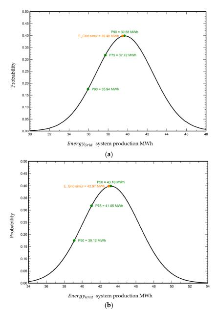
Figure 10. Probability distribution for (a) fixed and (b) tracking PV modules.
