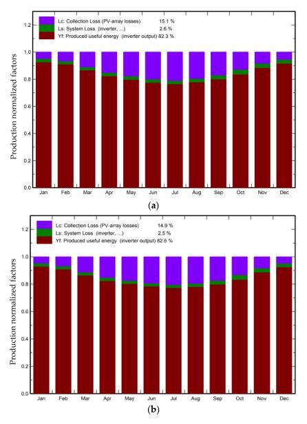
Figure 11. Normalized production and loss factors (a) fixed and (b) tracking systems.
