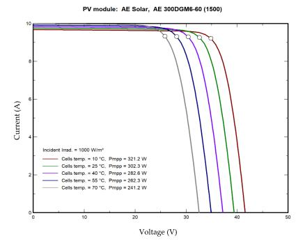
**Figure 2.** I-V graph for the used *PV* module under different temperature conditions (Obtained from *PV*syst software).
