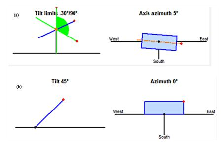
Figure 5. The orientation used, (a) tracking horizontal axis E–W and (b) fixed tilted plane.
