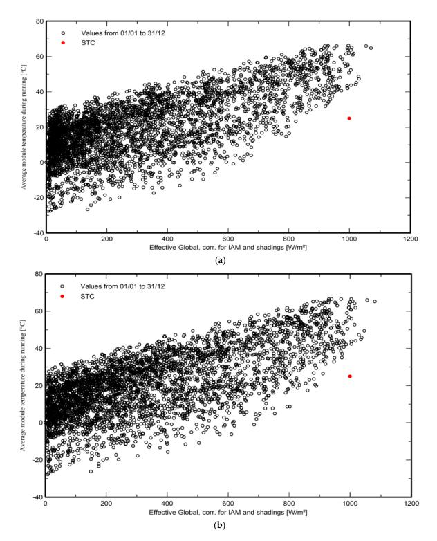
Figure 8. Array temperature vs. effective irradiance (a) fixed plane and (b) tracking PV system.
