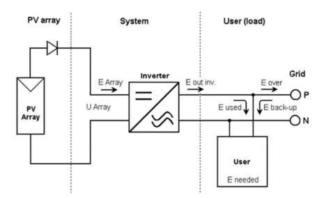
Figure 4. Schematic diagram of the proposed PV system.
