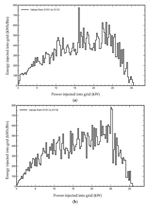
Figure 9. System output power distribution (a) fixed plane and (b) tracking system.
