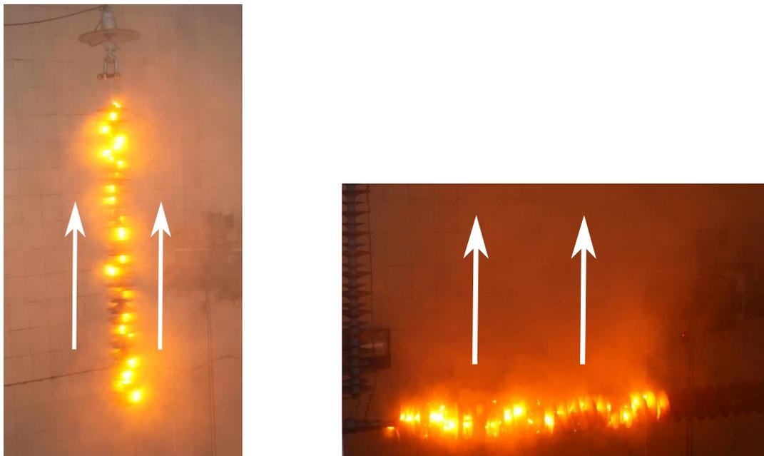
Fig. 3.13. Water vapour moving upwards during HVDC pollution flashover in both vertical, on the left, and horizontal, on the right, orientations.
