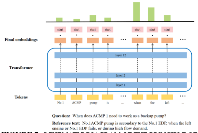
FIGURE 7: SCHEMATIC DIAGRAM OF THE PRINCIPLE OF THE BERT MODEL
