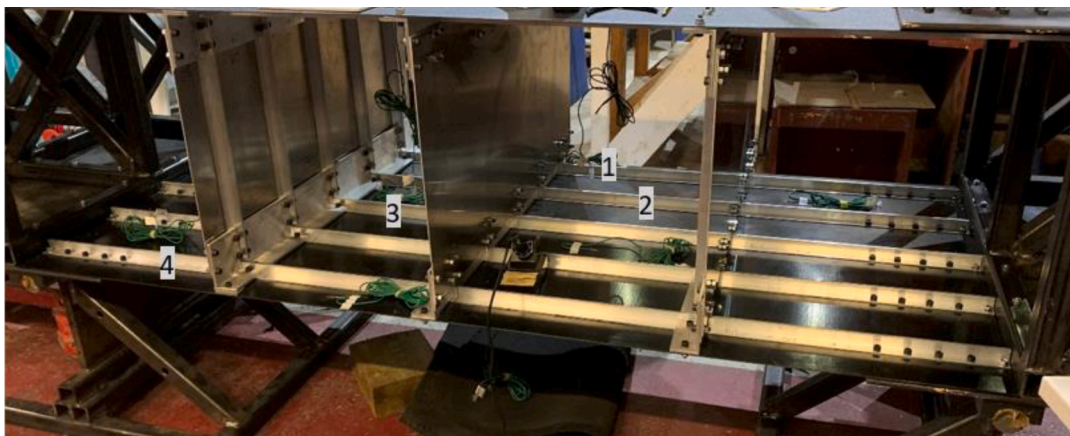
Fig. 13. Location of debonded stiffeners.
