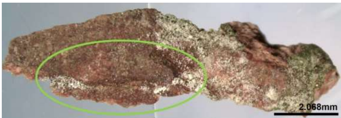
Figure 250: The surface of S21. Brown resinous substance is visible underneath deposits (circled).
