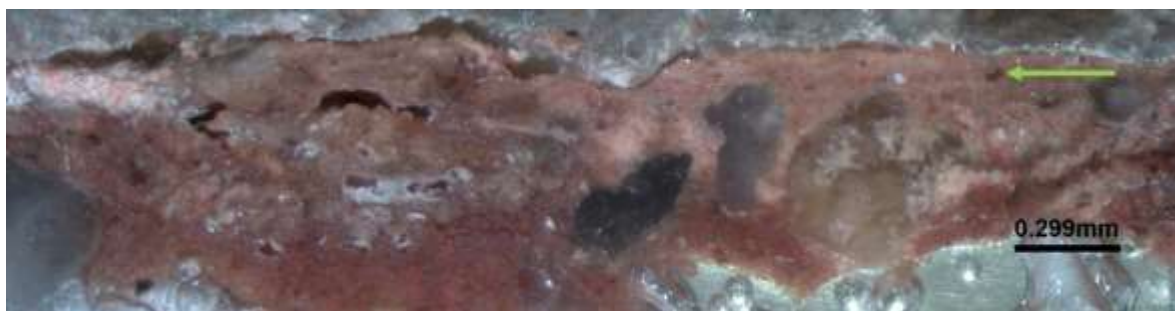
Figure 217: The cross-section of S10 showing a fine surface layer of calcite covered by thin white crust.
