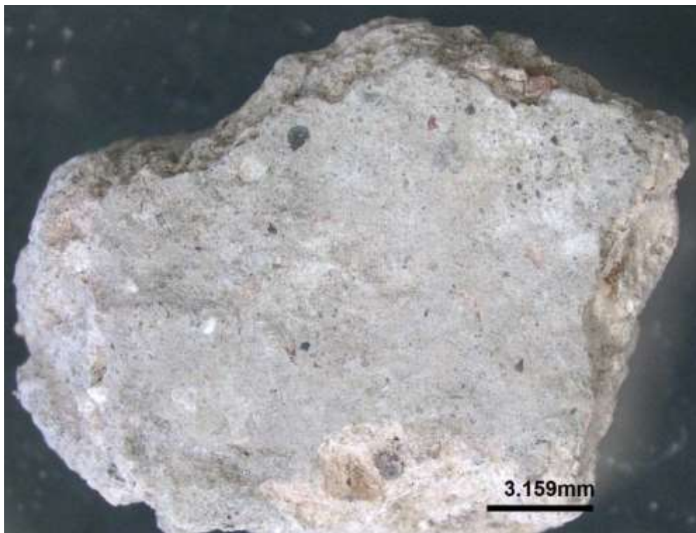
Figure 170: The surface of S4 appears grey and dense.
