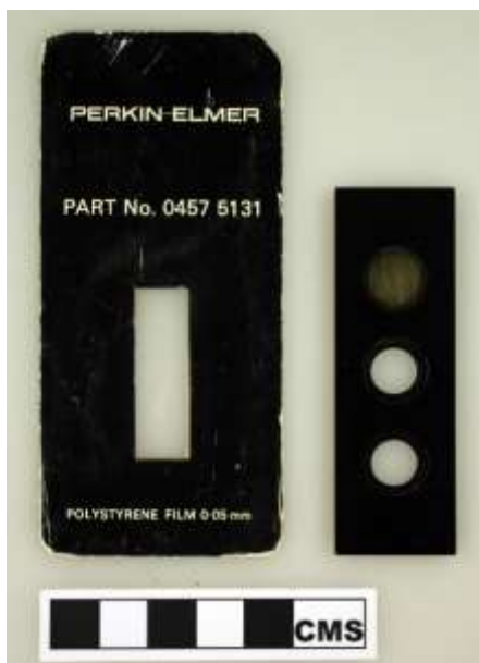
Figure 13: The Polystyrene film (PE) standard and the golden mirror for the background correction.
