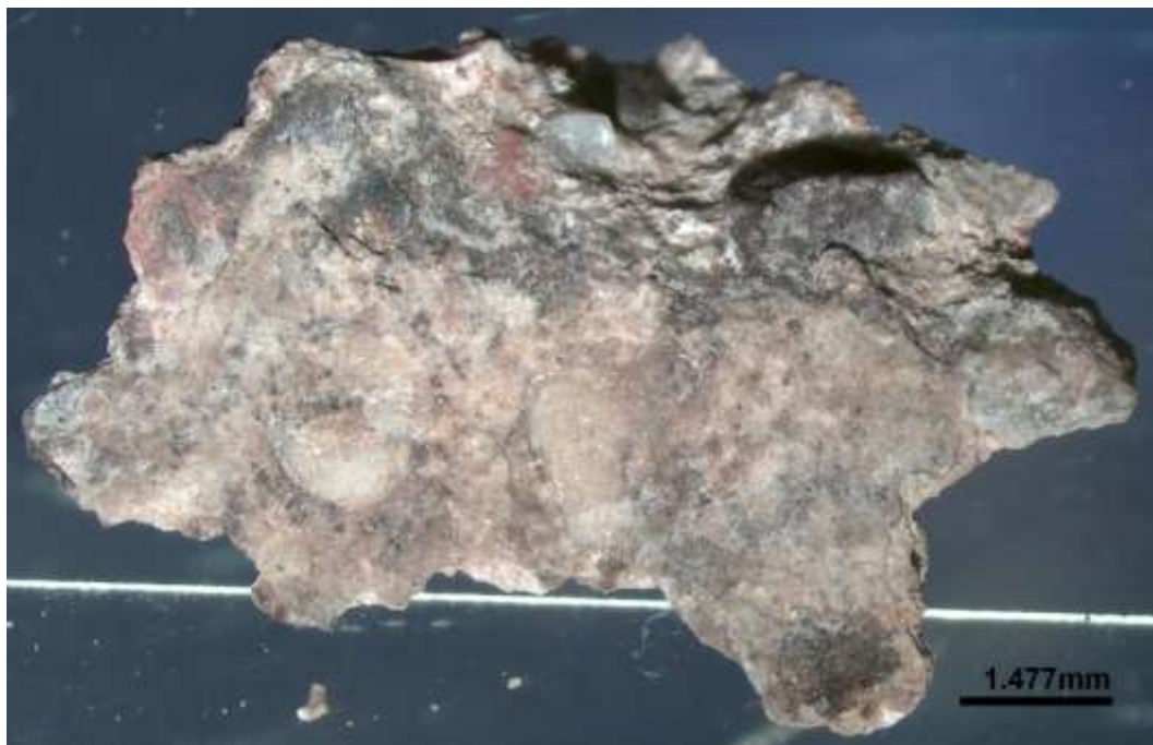
Figure 189: The flat surface of sample S15a showing accumulation of calcium carbonate deposits.
