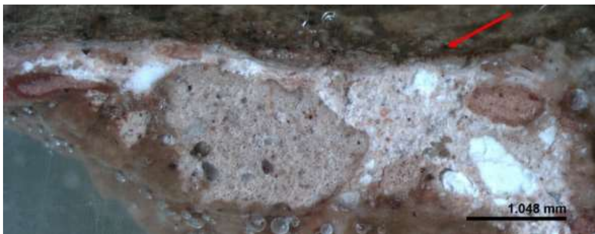
Figure 159: The cross-section of sample S2. Arrow points on the brown resinous substance on the flat surface.
