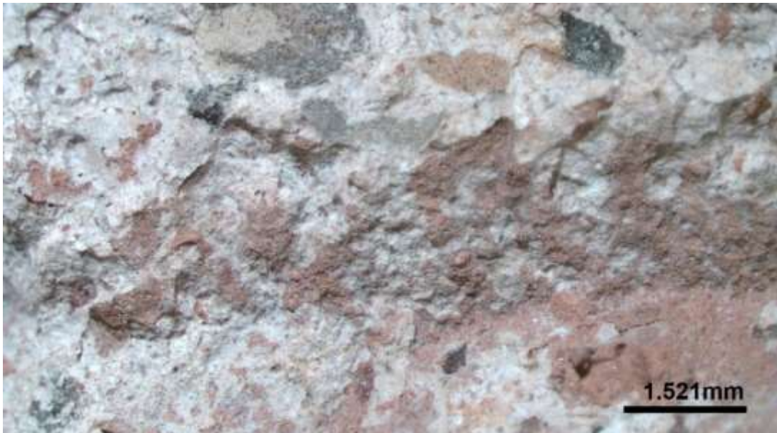
Figure 208: S13 mortar sample of the lime-quartz-crushed ceramic type.
