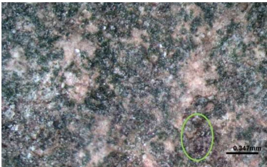
Figure 245: The surface of S20. Resinous deposits (circled) exist within a variety of other loose deposits.
