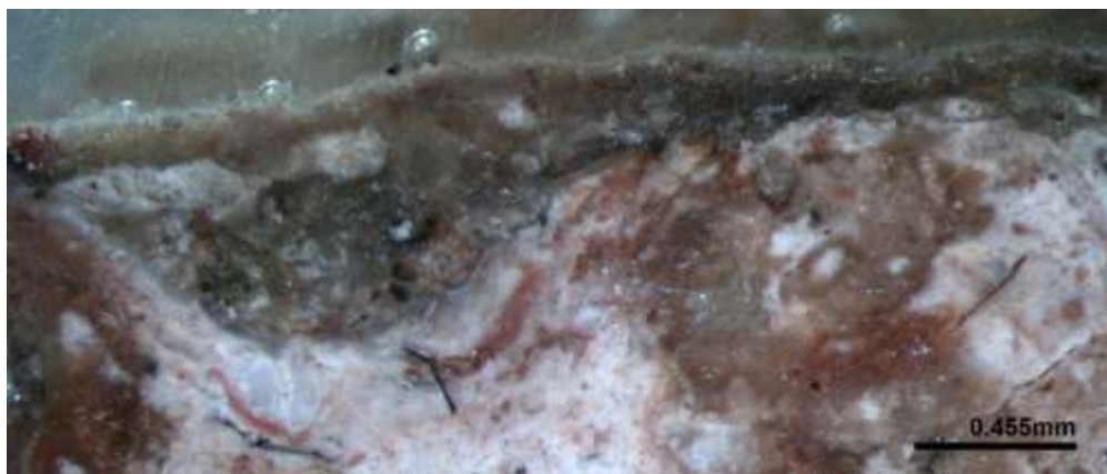
Figure 171: Cross-section of S4 showing a thick light brown to grey surface layer.
