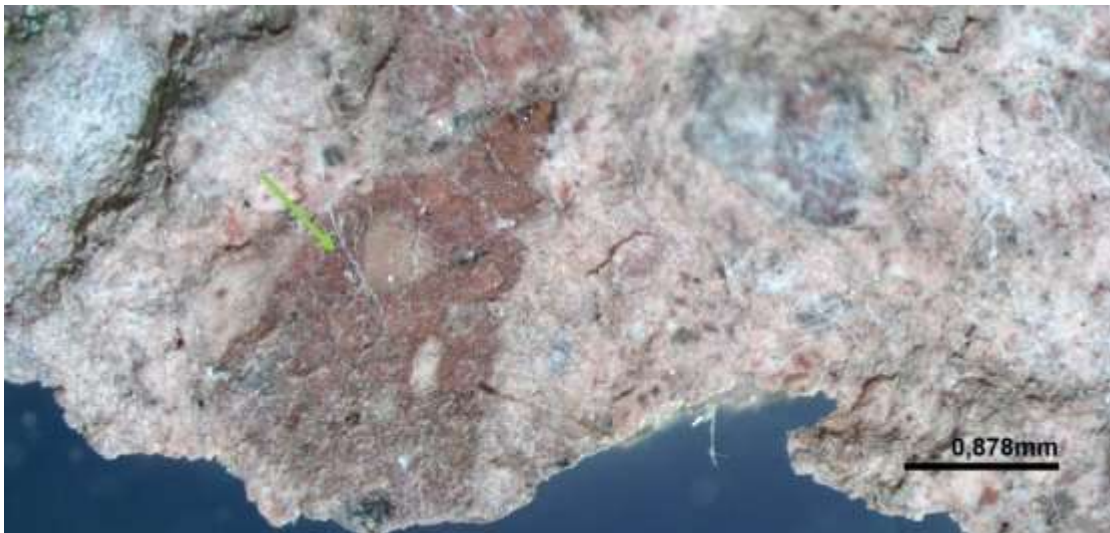
Figure 279: The weathered surface of S28; hyaline mycelium growth is indicated by the arrow.
