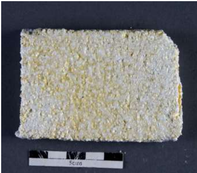
Figure 85: Mortar replica coated with egg yolk.
