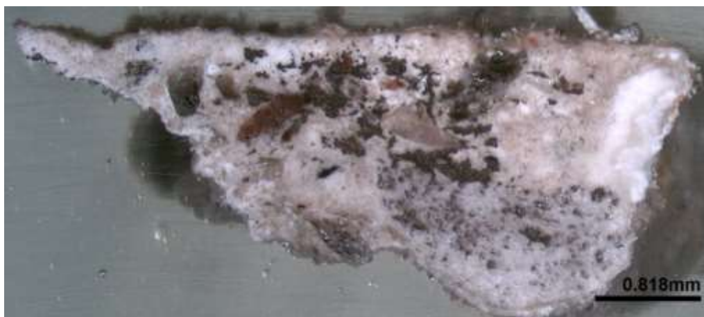
Figure 255: The cross-section of S22. The mortar consists mainly of lime and quartz.
