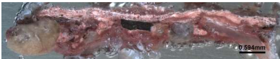
Figure 213: Cross-section of S8. The thick white crust covers the entire surface.
