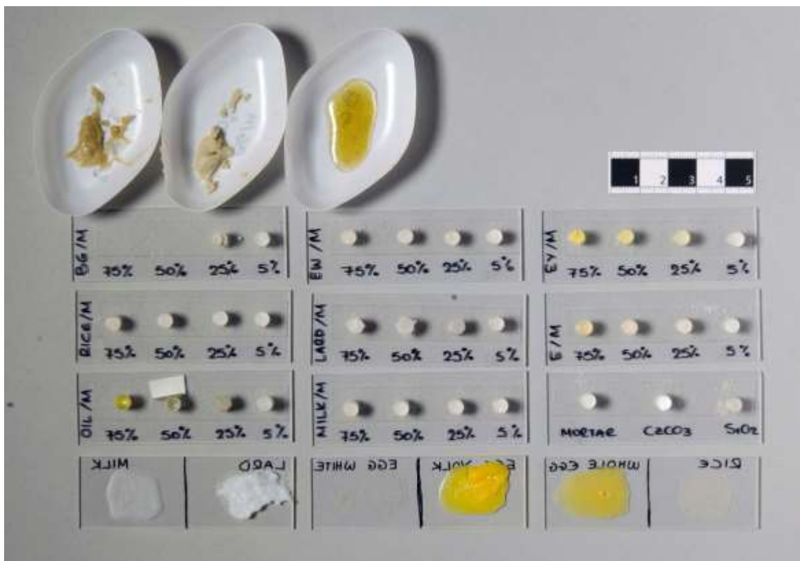
Figure 34: The laboratory prepared standards: films of organic materials, inorganic powders, mortar powder and organic/mortar mixtures.
