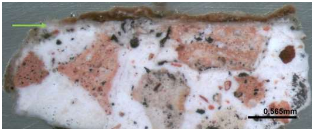
Figure 233: The cross-section of S18. Green arrow points to a fine white surface layer under brown patina.
