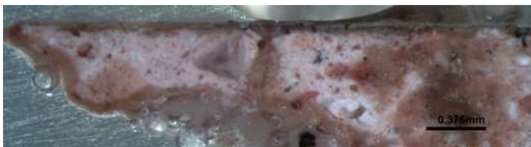
Figure 176: The cross-section of S5 showing a thin grey surface layer.
