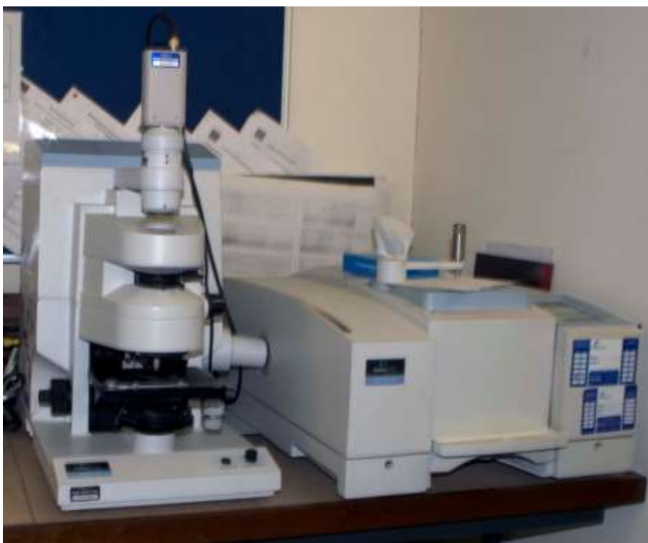
Figure 12: The FTIR microscope and spectrometer.
