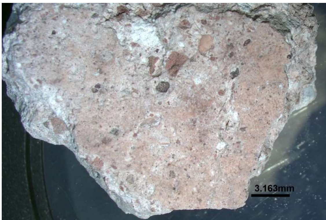
Figure 222: The flat surface of S12 appears light red to pink.
