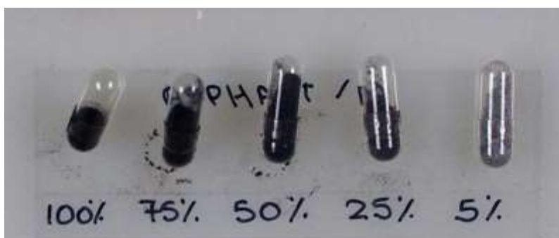
Figure 35: The standards of asphalt in gelatine capsules: 100% asphalt and asphalt/mortar mixtures in 75%, 50%, 25% and 5% organic concentration.
