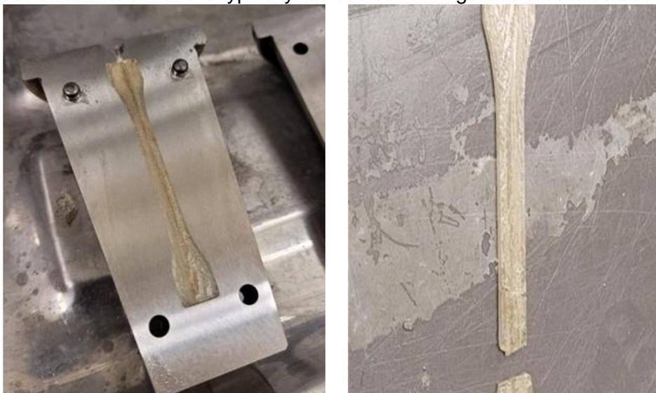
**Figure 4.23:** Images of extruded polymer showing the high crystallinity and brittleness of the extruded material.
