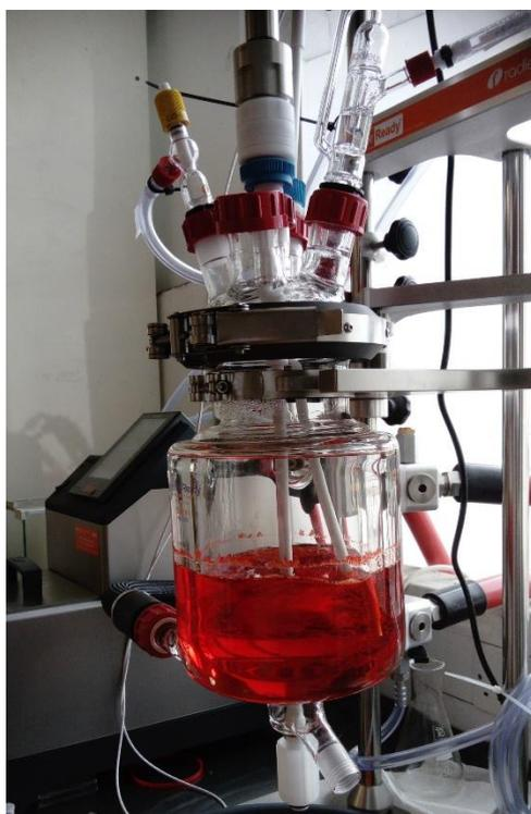
**Figure 4.10:** 2 litre reaction vessel used for large scale polymerisation reactions (**AAQ-PHA-CHO3**).
