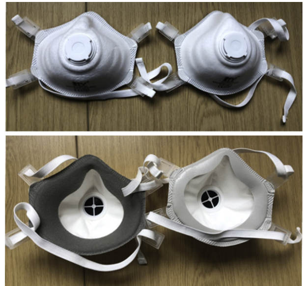
Figure 5 Differences in the inner seal of the same FFP3 Handanhy 9632 mask.
