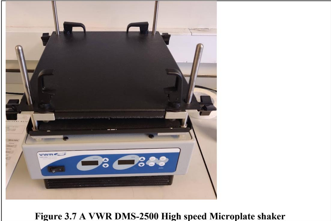
**Figure 3.7 A VWR DMS-2500 High speed Microplate shaker**
