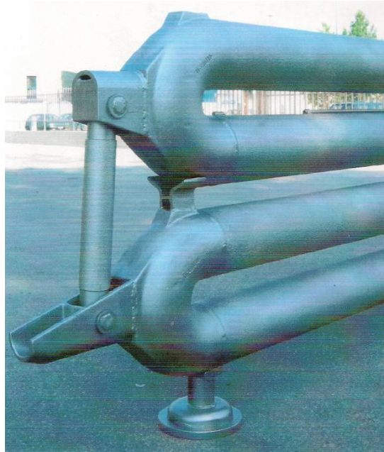
Figure 4-11 - New support design adopted by Segal, where the top return bend is supported by the lower support via a tubular link/rod
