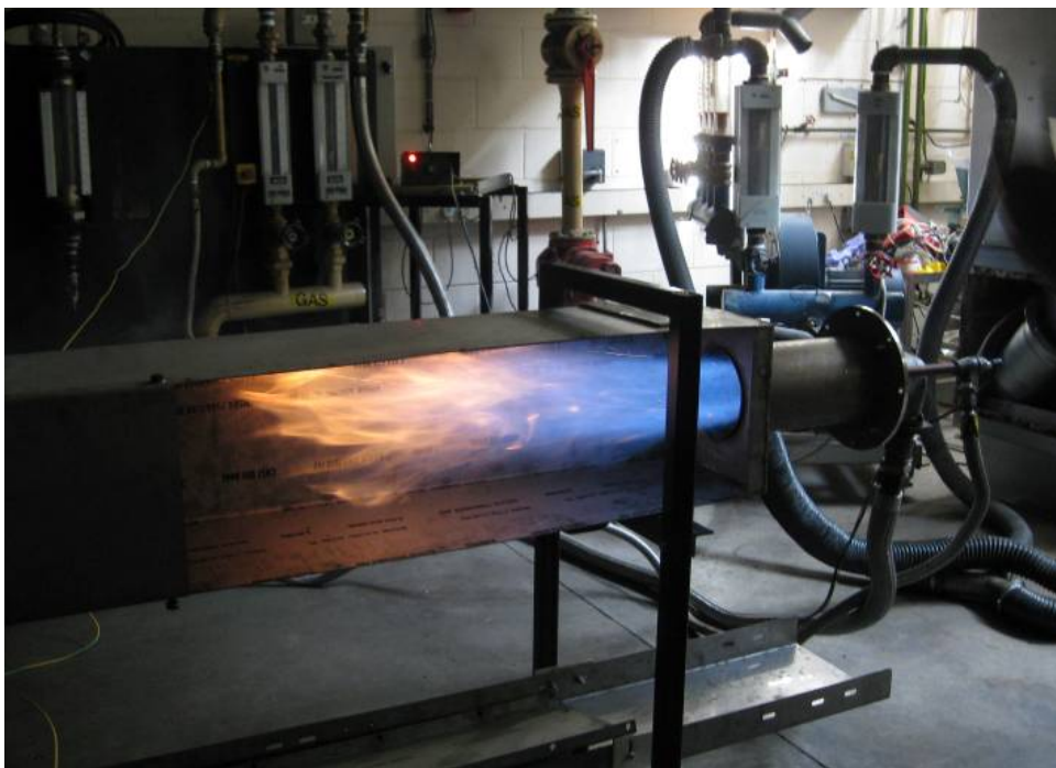
Figure 8-8 - Problems with lighting the main burner were experienced during preliminary tests
