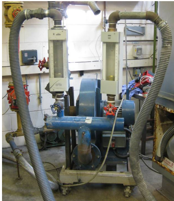
Figure 8-3 - Electric fan fitted with rotameters, capable of delivering 4500L/min of air
