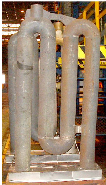
Figure 4-1 - Radiant tube design used at the CAPL at Trostre Works
