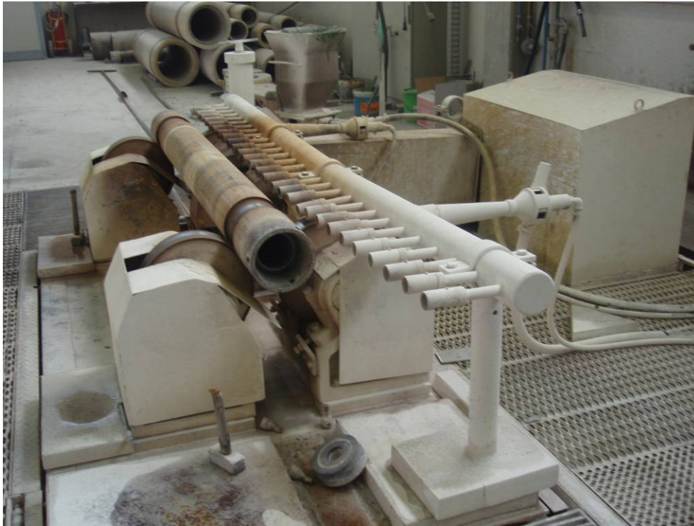
Figure 2-11 - Image showing a spin-casting machine able to produce cast tubes. Note different size moulds in background to produce various diameters of tubes
