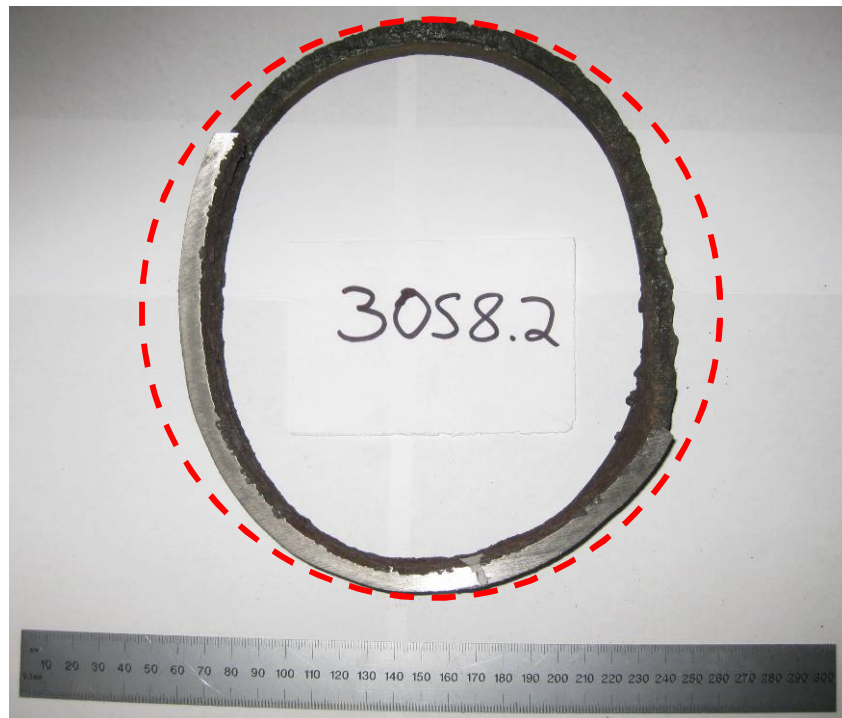
Figure 6-4 - Very low levels of deformation visible in weld failure samples
