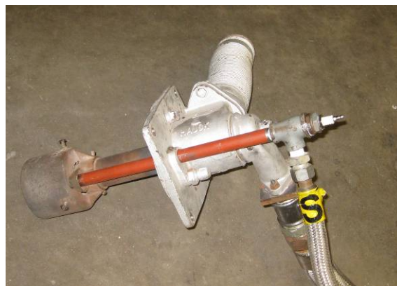
Figure 8-5 - Natural gas burner fitted with pilot burner for main burner ignition
