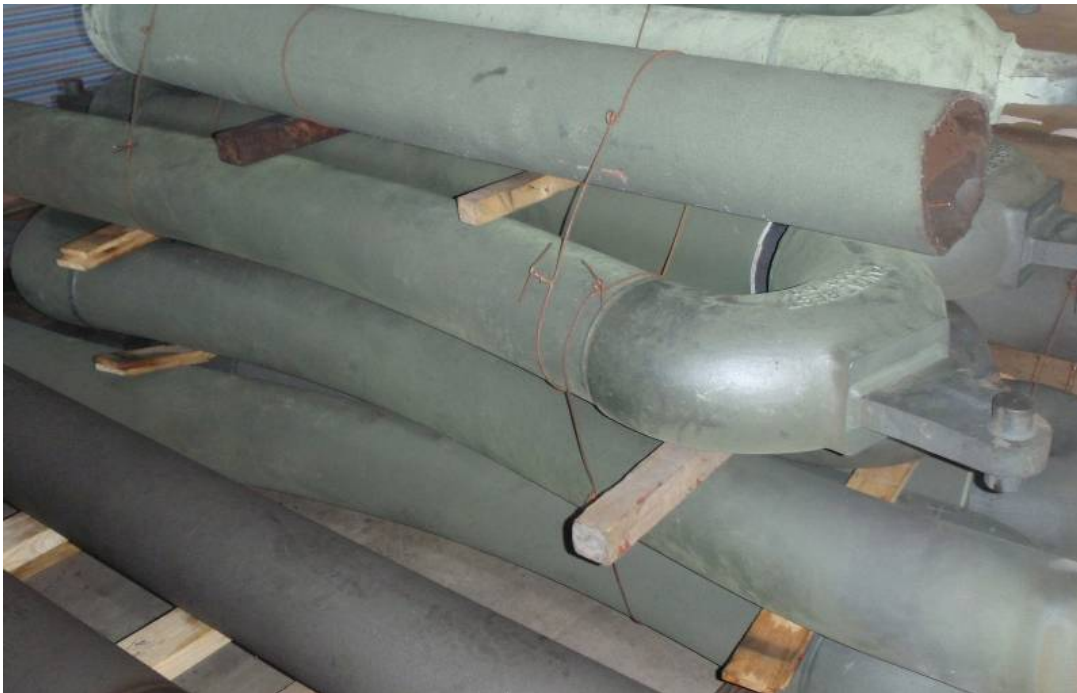
Figure 4-19 - Failed radiant tubes showing signs of deformation in the firing and second leg
