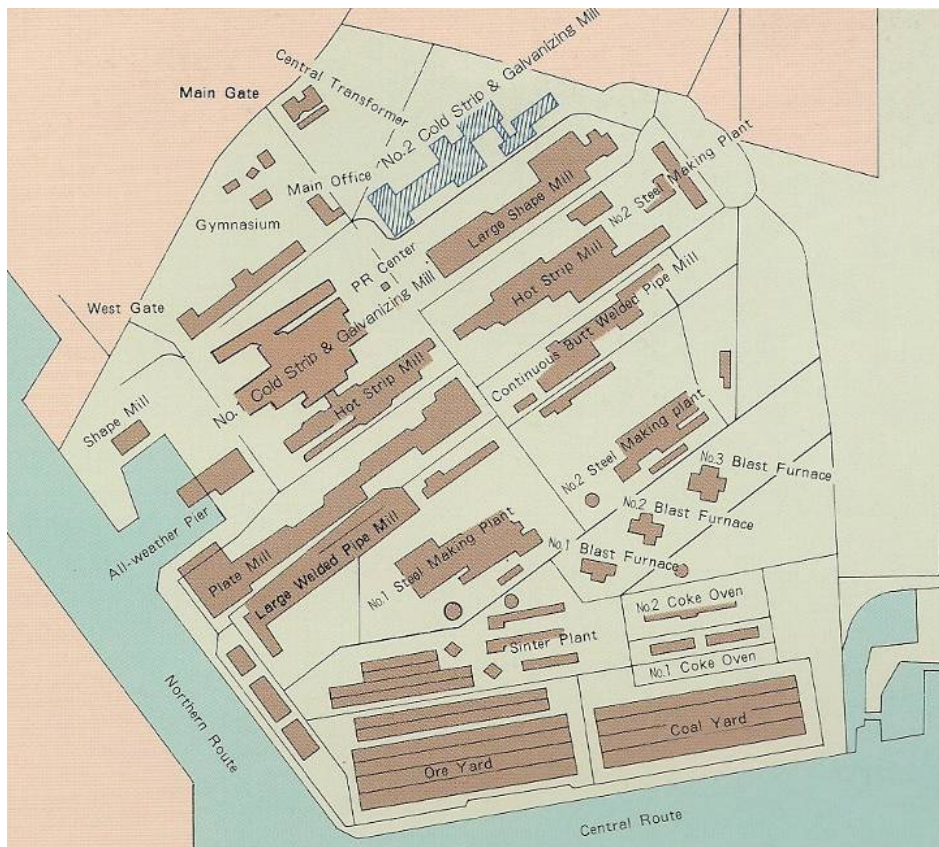
Figure 4-15 - Plant Layout of Kashima Steel Works
