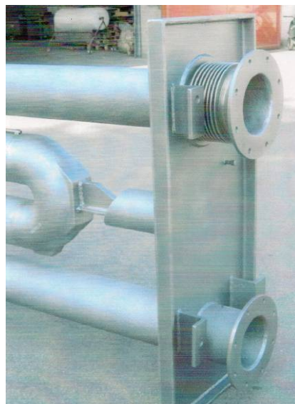
Figure 4-9 - Bellows fitted to the firing leg of the Segal radiant tube allowing expansion along the length of the tube
