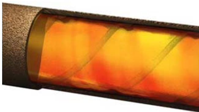
Figure 9-1 - Image displaying a section of a MERT radiant tube showing the continuous weld bead on the inside of the tube surface 79
