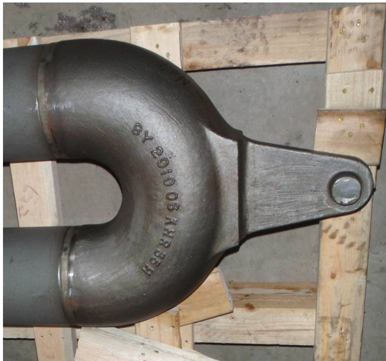
Figure 4-21 - New bend support design aimed at reducing the bending force in the tube
