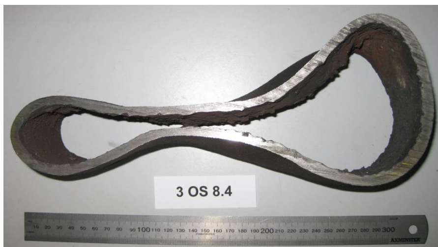
Figure 6-7 - Severe deformation of firing leg leading to cracking (not shown)
