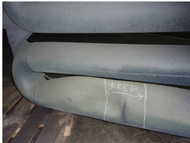
Figure 6-2 - Example of deformed firing leg, which has resulted in a crack
