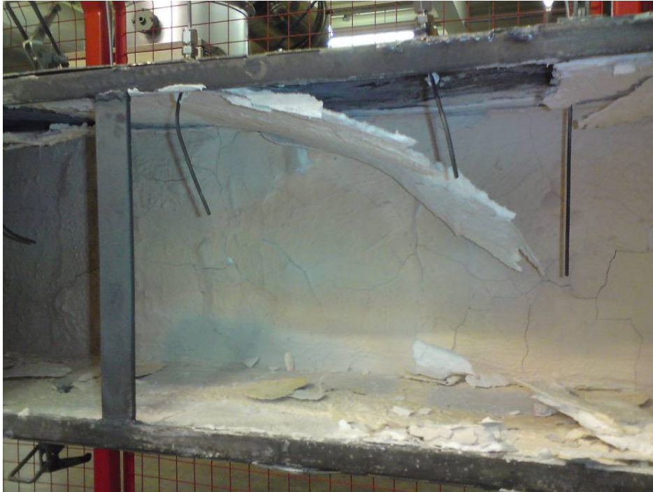
Figure 8-9 - The thermal lining cracked, distorted and worked loose from the Inconel structure during thermal cycling experiments
