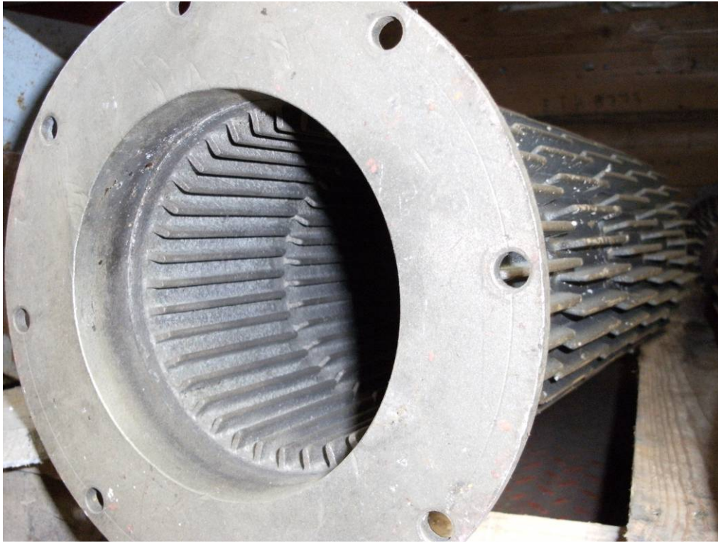
Figure 2-3 - Recuperator heat exchanger recovering heat energy from the hot exhaust gases and transferring them to the incoming combustion air
