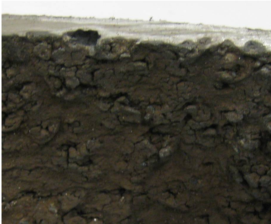
Figure 6-16 - Example of how the oxide layer breaks up and cracks and eventually breaking off exposing fresh metal underneath to further oxidation
