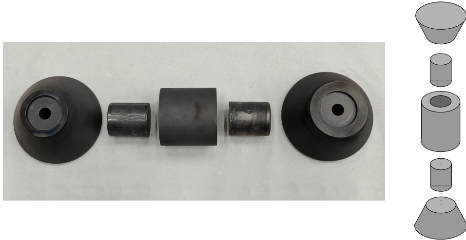
Figure 3.9: Exploded view of the graphitic die assembly for 30 mm samples.
