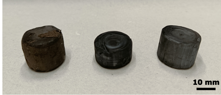
Figure 4.30: Visual comparison of thermally reduced aerogels. Left: 0.5:CU\_rGO_{ag} . Middle: 0.5:CU\_GO_{ag}(0.02N) . Right: 0.5:CU\_GO_{ag}(0.05N) .
