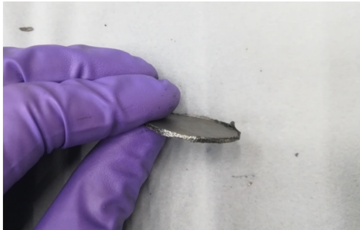
Figure 6.12: 30 mm discs after SPS of scaled-up 25:\text{Al}_2\text{O}_3/0.5:\text{ICL\_rGO}_{ag}\perp green bodies.
