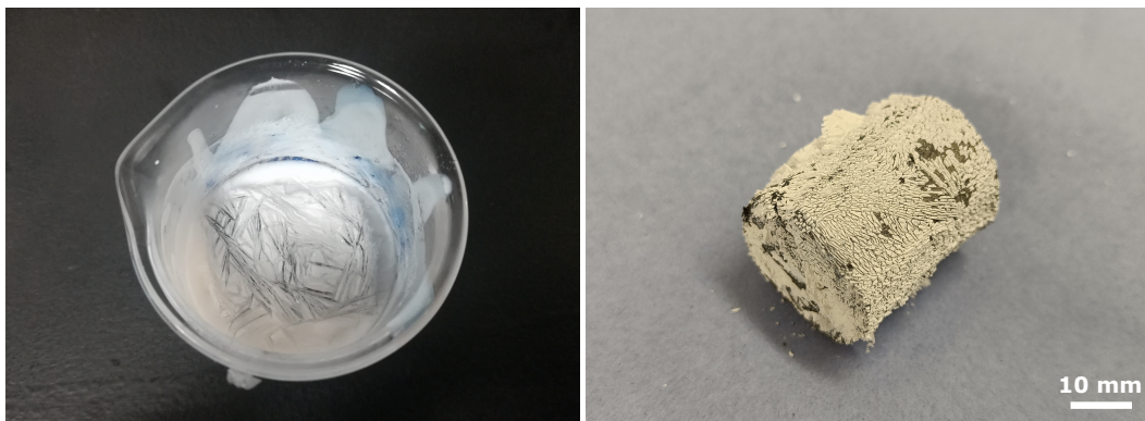
Figure 5.27: Infiltration and freeze-drying of scaled-up 0.5:ICL_rGO ag aerogels.
