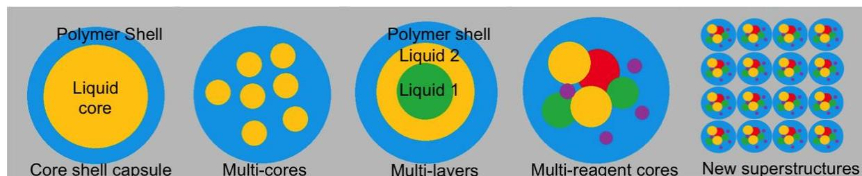
*Figure 1: Schematic of core-capsule structures of varying complexity.*
