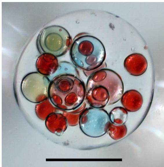
Figure 6: Photocured polymer capsule containing 4 different reagent solutions within different sized aqueous cores. The scale bar indicates 500 $\mu$ m.
