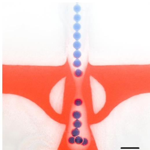
Figure 3: Image of double emulsion formation within the ‘bat-wing’ junction. Blue=potassium carbonate + thymol blue; white=NOA 61; Re=mineral oil + oil red O. Scale bar =500um
