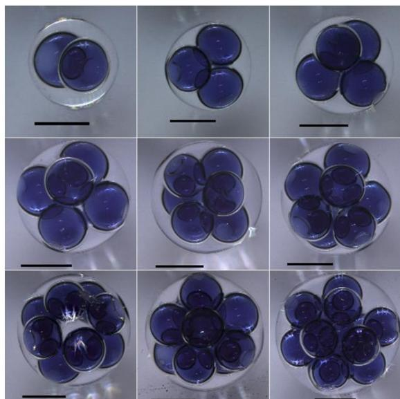
Figure 5: Photocured polymer capsules with defined numbers of aqueous inner cores, each of a defined volume. From top to bottom, left to right, inner cores number sequentially, 2-10. All scale bars indicate 500 $\mu$ m.
