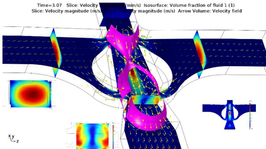
Figure 2: COMSOL simulation of droplet breakup; velocity magnitudes of fluid flow at different cross sections, indicated. Purple film indicates the isosurface between the dispersed and continuous phases; yellow arrows show local flow direction, their size presenting the velocity magnitude in a logarithmic scale.
