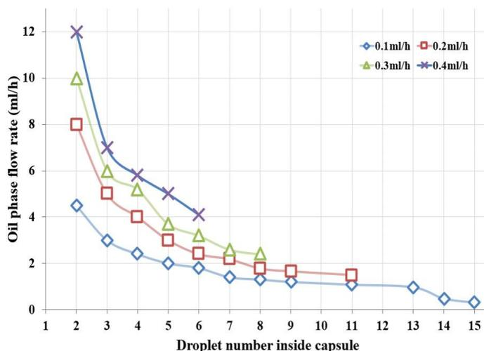
Figure 4: The relationship between droplet number and oil phase flow rate. Here, the aqueous and polymer phases have a constant flow-rate ratio. Aqueous phase flow rates are labelled.
