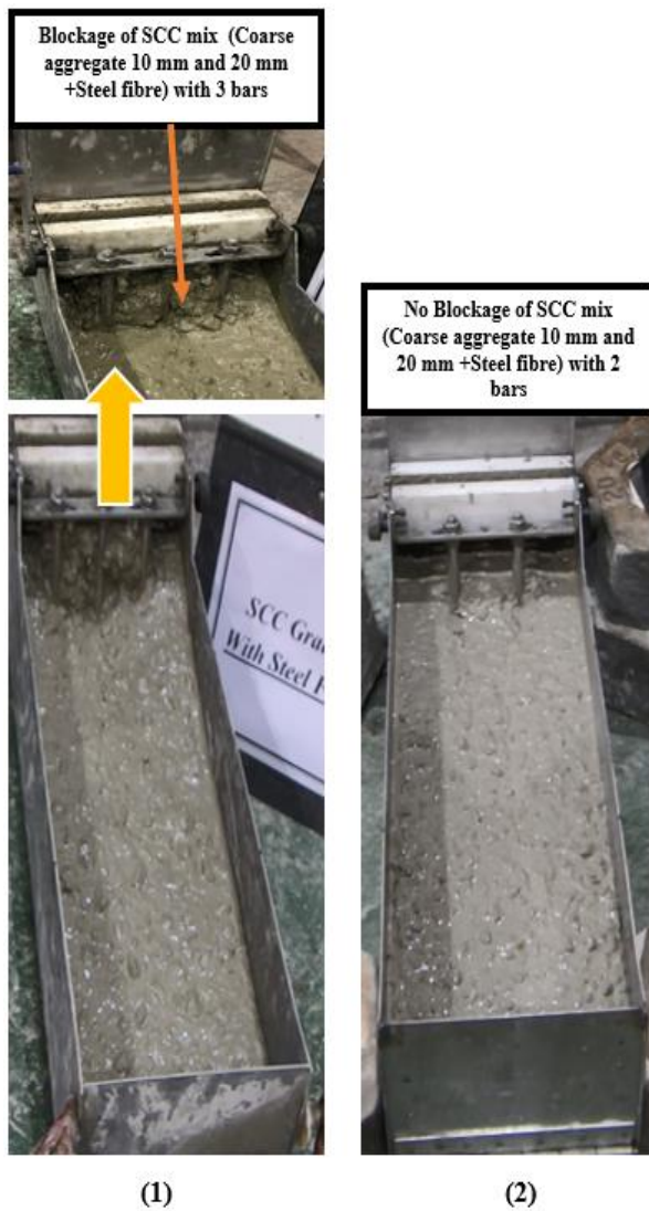
Figure 3: Flow, passing and filling ability of SCC and SCSFRC mix: C40 (1) with 3 bars, C40 (2) with 2 bars
