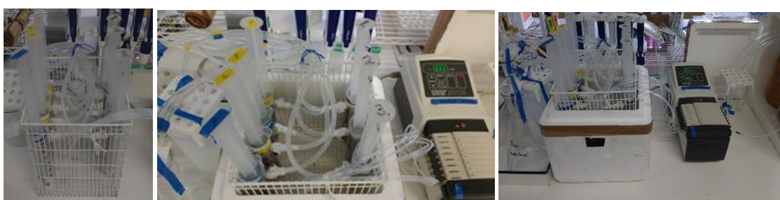
Figure 3.3. Photographs of the syringe sand columns with single-pass flow system for loading biofilm ( Bacillus mojavensis grown in Nutrient Broth E).
