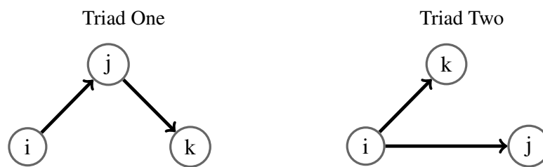
Figure 1.3: Different roles edges can play in connected triads. In Triad One, the edge (i, j) can support flooding the triad, but it does not in Triad Two. In Chapter Four we define edges as overt or covert, where in this example (i, j) acts as overt in Triad One and covert in Triad Two. Were this to represent communication on edge (i, j) , then when (i, j) is overt (Triad One).
