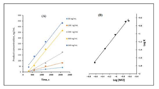
**Figure 6.** (**A**) Product concentration (ng/mL) versus time (seconds) curve for increasing concentrations of NFZ, and (**B**) log K versus log [NFZ] curve.
