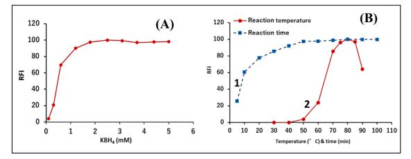
**Figure 3.** Effect of **(A)** concentration of the reducing agent, potassium borohydride, **(B)** the reaction time (1) and temperature (2) on the relative fluorescence intensity of the reduced NFZ.
