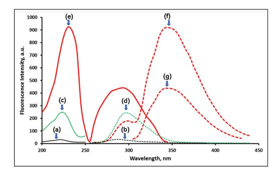
**Figure 2.** Excitation and emission spectra of NFZ alone (a, b), blank reducing agent (c, d), and reduced NFZ (e, f, g), where f and g represent reduced NFZ emission spectra after excitation at 230 and 295 nm, respectively. The excitation spectra are presented as solid lines, and emission ones are presented as dashed lines.
