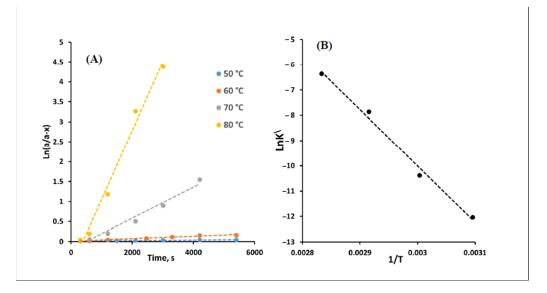
**Figure 7.** (**A**) Semi logarithmic plot for the first-order reaction of NFZ and potassium borohydride and (**B**) Arrhenius plot for the reaction of NFZ and potassium borohydride.
