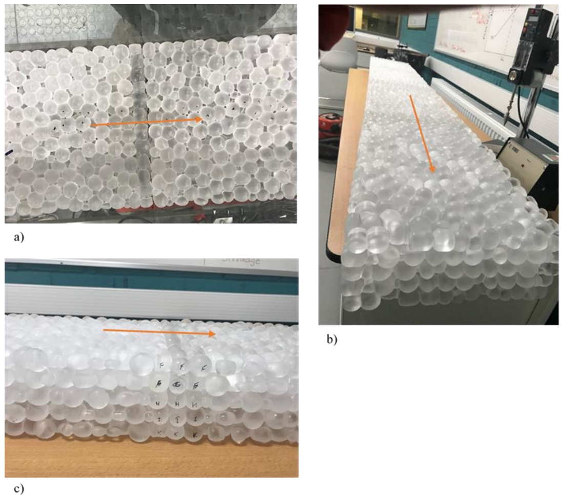
Figure 3.4. The artificial bed a) a top-view sectional view in the x-y plane, b) a cross-sectional view in the z-y plane, and c) a streamwise sectional view in the x-z plane. The flow direction is indicated by the arrow in each figure.
