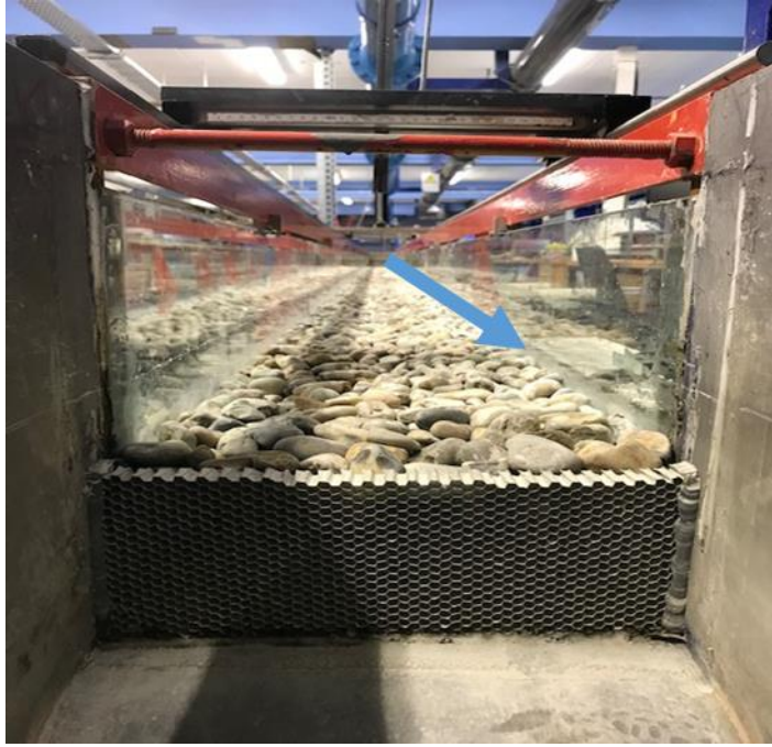
Figure 3.10. An image of the flume outlet looking in the upstream direction, showing the honeycomb lattice in place, preventing gravel particles from entering the outlet tank whilst allowing flow through the subsurface region. The flow direction is indicated by the arrow.
