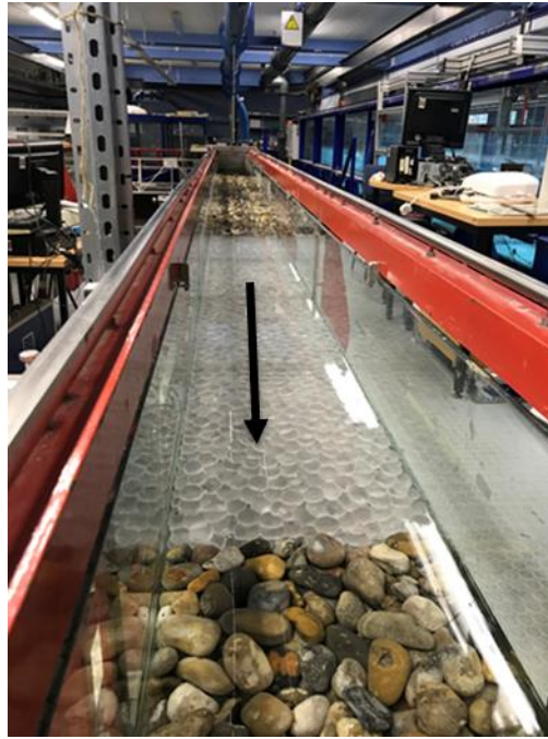
Figure 3.6. A novel artificial bed with a median particle diameter of 28 mm was placed within the test section for experiments 5 and 6.
