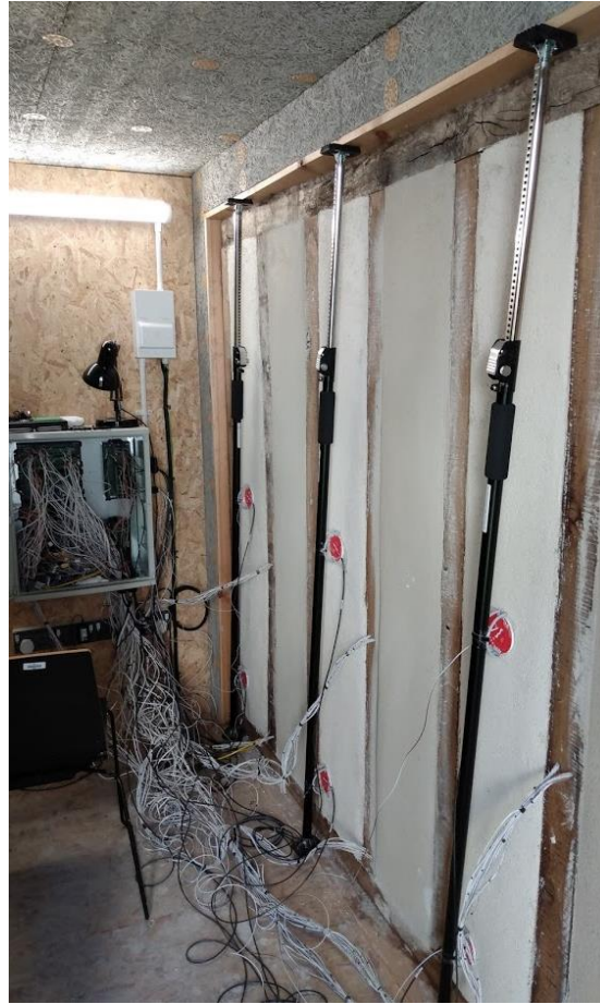
Test panels completed onsite by Royston Davies and UK Hempcrete.
