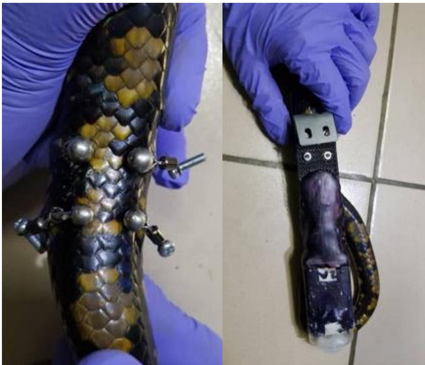
*Figure 3.4* A later development during phase 3, placing two piercings frontally, and securing them to the unit using screws and fishing swivels, rather than wire. The VHF and GPS logger have been placed within a far stronger housing, attached to flexible belting.
