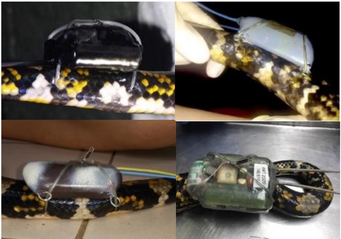
**Figure 3.1** Phase 1 tags after attachment to python tails. The Telenax unit is top left, while the other three were manufactured by AWT.
