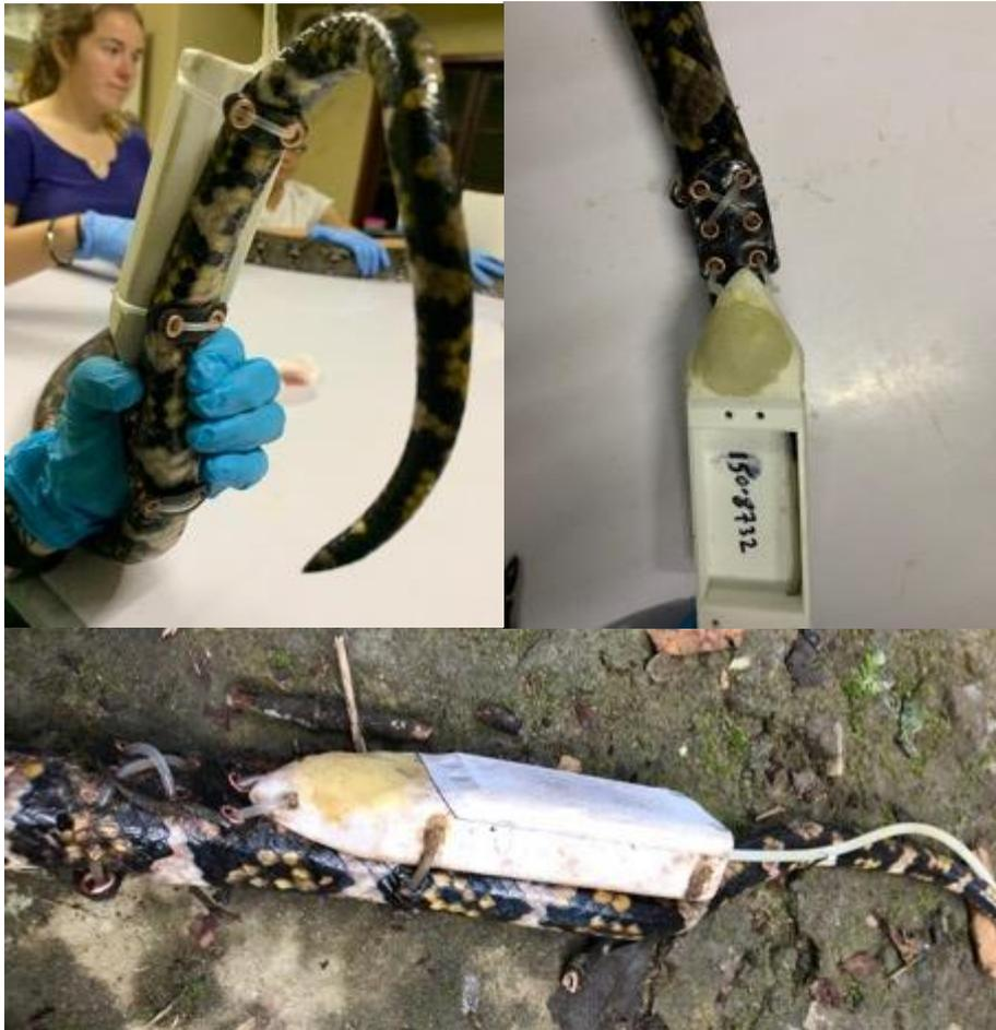
**Figure 3.5** Highlighting Phase 4 tag casing design and attachment. The anterior attachment consisted of a “saddle” intended to spread any forces created by the tag being caught on vegetation. Epoxy spacers were used ventrally with the wires to further reduce any force on a single location. GPS loggers could be quickly replaced within the casing by unscrewing the lid.
