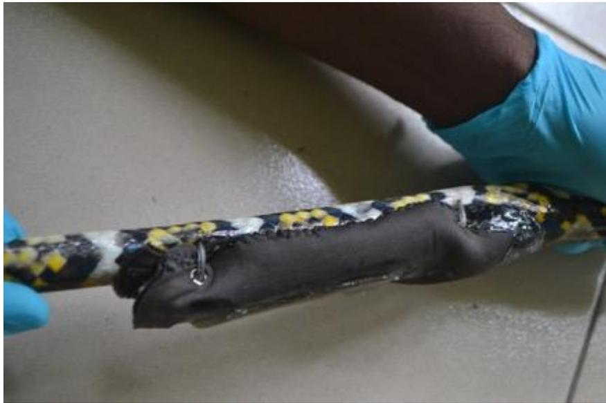
**Figure 3.2** *Prototype flexible neoprene pouch design used in phase 2. The top and front can be seen to be reinforced with epoxy resin.*
