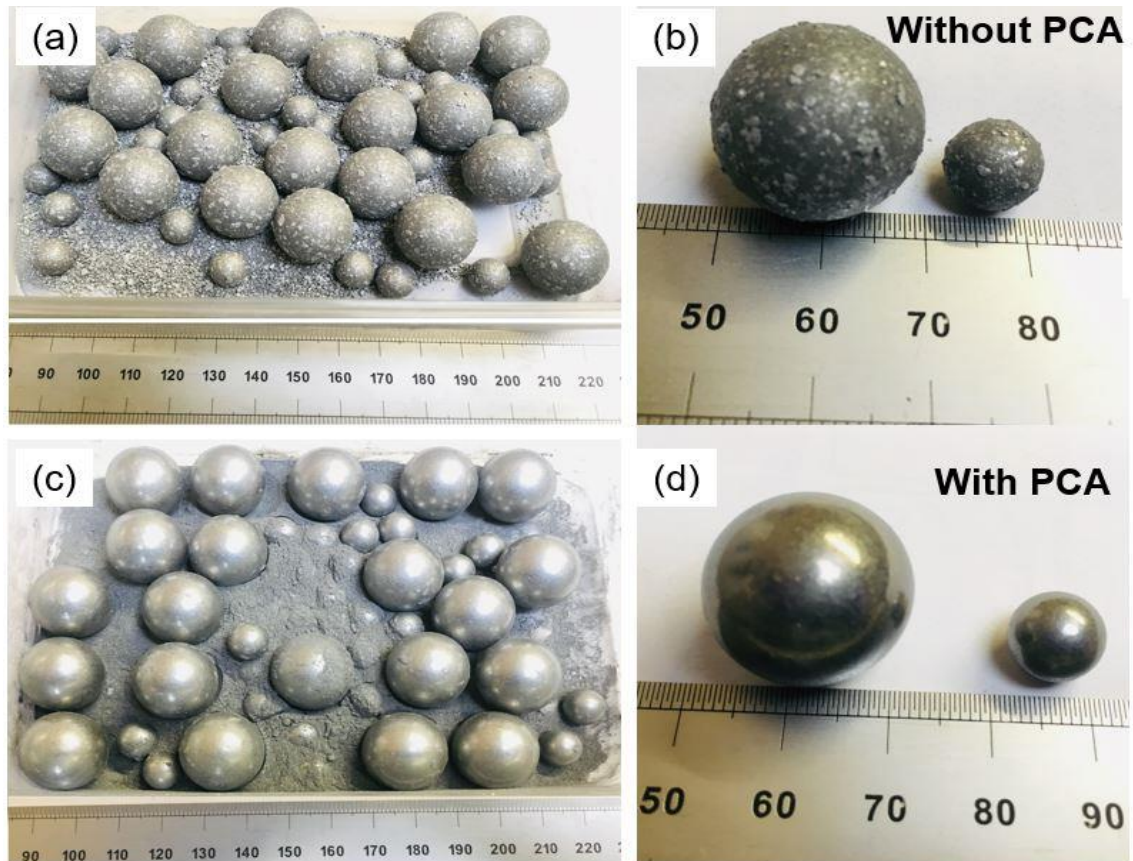
Figure 5.1: The milling balls and powder after 15 minutes of milling without (a-b) and with 2% of PCA (c-d).
