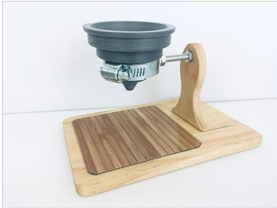
Figure 3.5 Powder flowability determination kit.
