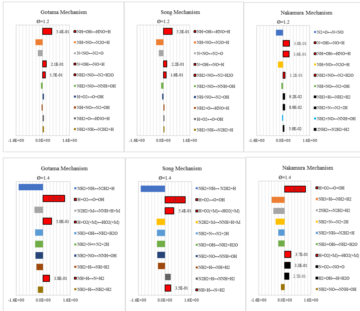
Figure 8: Sensitivity analysis for laminar flame speed of 70NH 3 /30H 2 (%vol) under atmospheric conditions and for three kinetic reaction mechanisms ( Gotama, Song, and Nakamura) that give a minimum discrepancy value at a rich range of equivalence ratio of 1.2 -1.4. Critical reactions for the laminar flame speed are marked in red colour.
