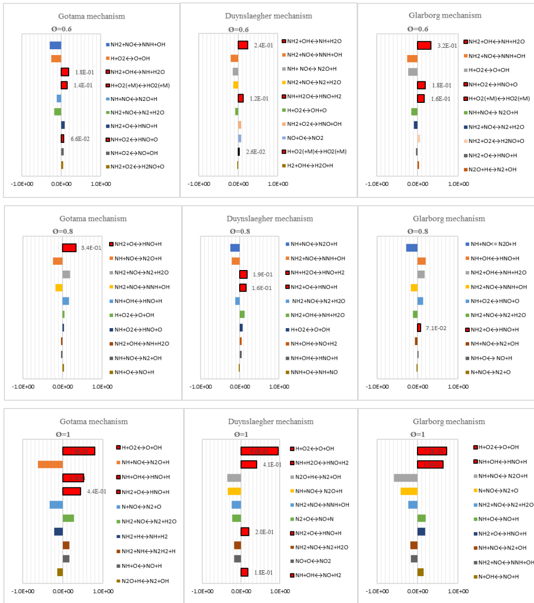
Figure 5: Sensitivity analysis for laminar flame speed of 70NH 3 /30H 2 (v/v%) under atmospheric conditions and for three kinetic mechanisms (Gotama et al. 2022, Duynslaegher et al. 2012, and Glarborg et al. 2018) that give a minimum discrepancy value at a lean range of equivalence ratio of 0.6-1.0. Critical reactions for the laminar flame speed are marked in red colour.
