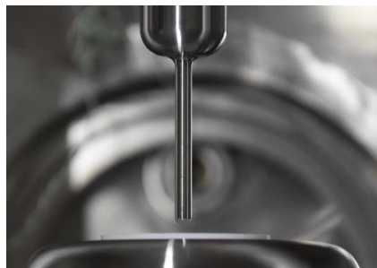
Fig. 10. Bright field image of rod – plane configuration with PTFE barrier
