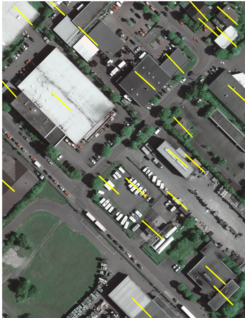
Figure 4.14: Resultant output image based on Method 2 finding building references, where a yellow line represents one of the buildings' orientations.
