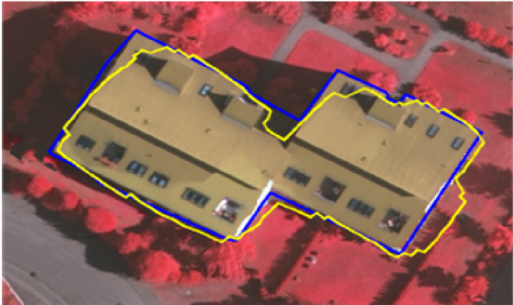
Figure 4.6: Previous result: the white line is post-processed contour (Method 1), yellow is predicted contour (SAGAN), and blue is ground truth.
