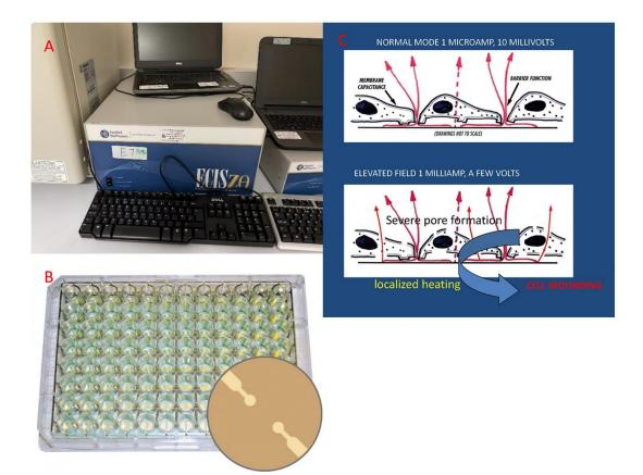
Figure 2.14 Electric cell-substrate impedance sensing system. A: The ECISZ $\theta$  unit used in the present study. B: The 96W1E electrode array used in the present study. (Applied Biophysics Inc., NJ, USA) C: Method to measure cell-substrate impedance (www.biophysics.com)
