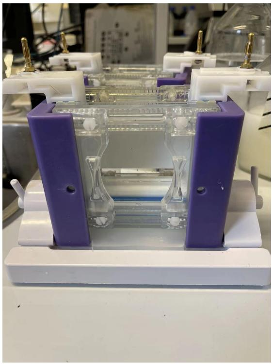
Figure 2.9 OmniPAGE VS10 vertical electrophoresis system (Wolf Laboratories, York, UK)
