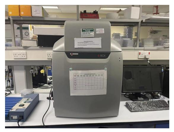
Figure 2.11 G:BOX Chemi XRQ protein detection system (Syngene, Cambridge, UK)
