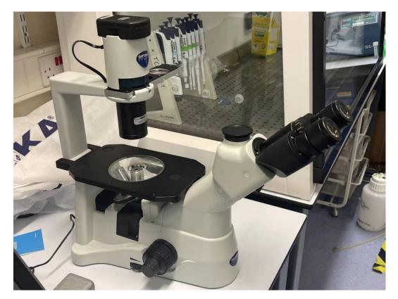
Figure 2.1 Inverted microscope (Leica Microsystems (UK) Ltd, Milton Keynes, UK).
