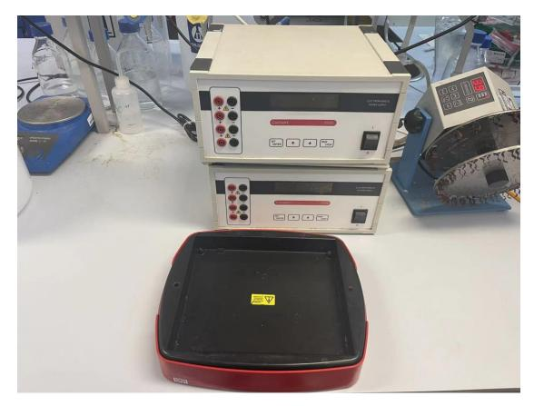
Figure 2.10 SD10 SemiDry Maxi System blotting unit (Wolf Laboratories, York, UK)
