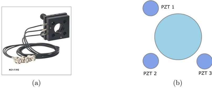
Figure 3.20: **a)** picture of the Thorlabs KC1-PZ(/M) steering mirror. **b)** the arrangement of the PZTs to control the tip/tilt of the steering mirror.
