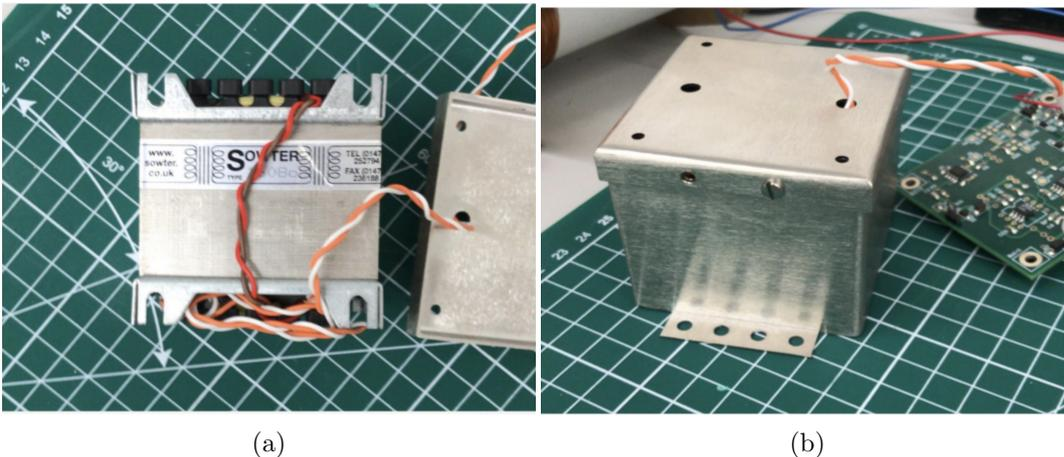
Figure 2.46: **a)** the original inductor prototype. The brown and red wires are optional taps at 2 H and 3 H respectively which are only present on this evaluation model. **b)** prototype mu-metal case that was used for testing. The new design shown in figure 5.11 was designed for two inductors, but has the same wall thickness of 1 mm.
