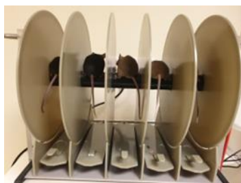
Figure 2.12: Rotarod apparatus. Up to 5 mice were tested simultaneously, a 300 second cut-off per trial was used.
