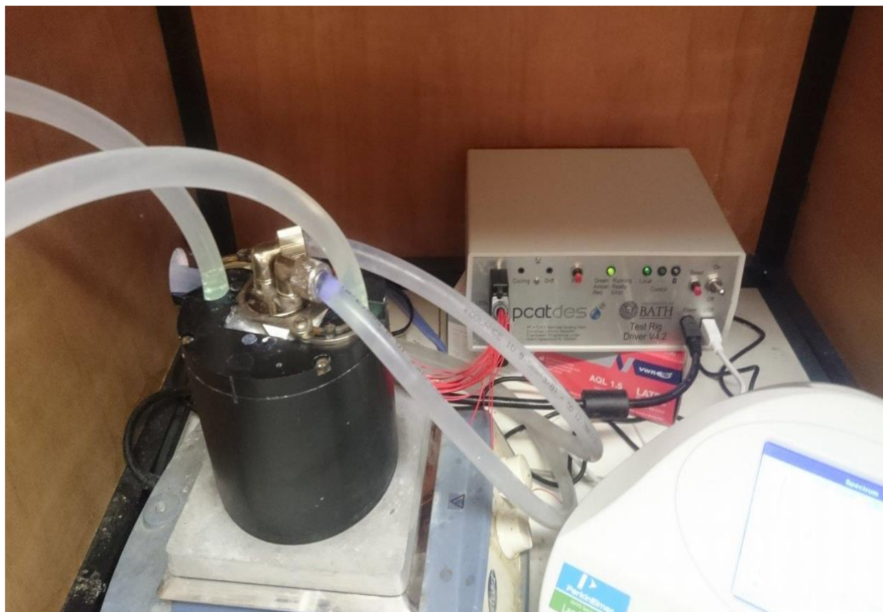
Figure 2-1 Reaction set up and Photoreactor (single wavelength)
