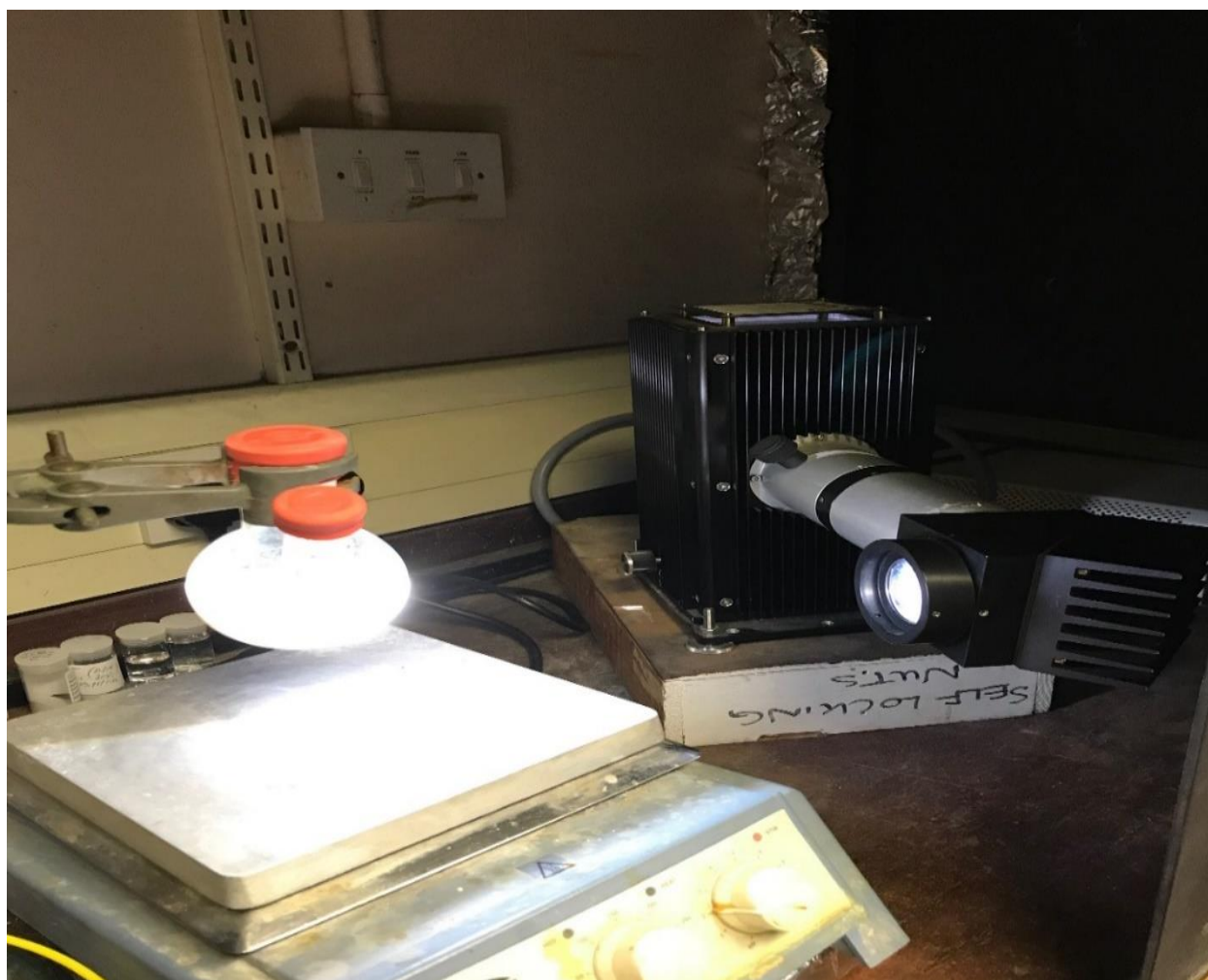
Fig. 2-2 Picture of xenon lamp and pyrex flask (photoreactor) containing mixture of deionized water, glycerol and Pt/TiO 2
