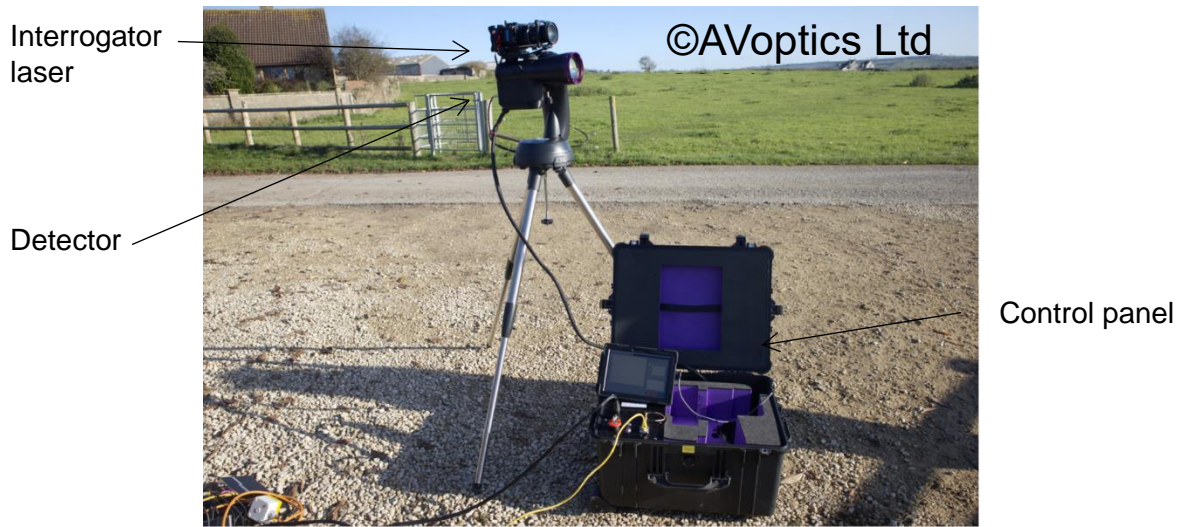
Fig. 1.1 – Free space optical transceiver station from AVoptics Ltd.
