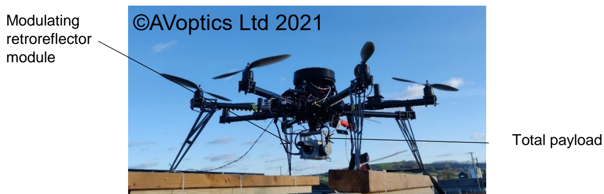
Fig. 1.3 – Octocopter drone with MRR for free space optical communication, from AVoptics Ltd.
