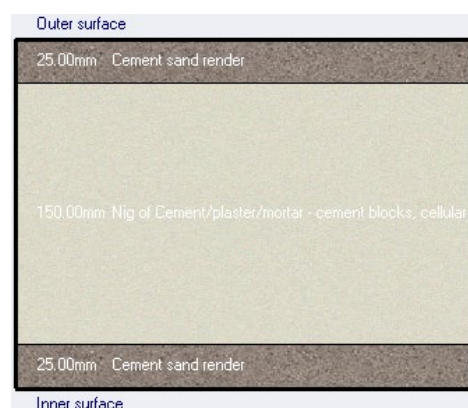
Figure 89: DesignBuilder Sandcrete layers representation
