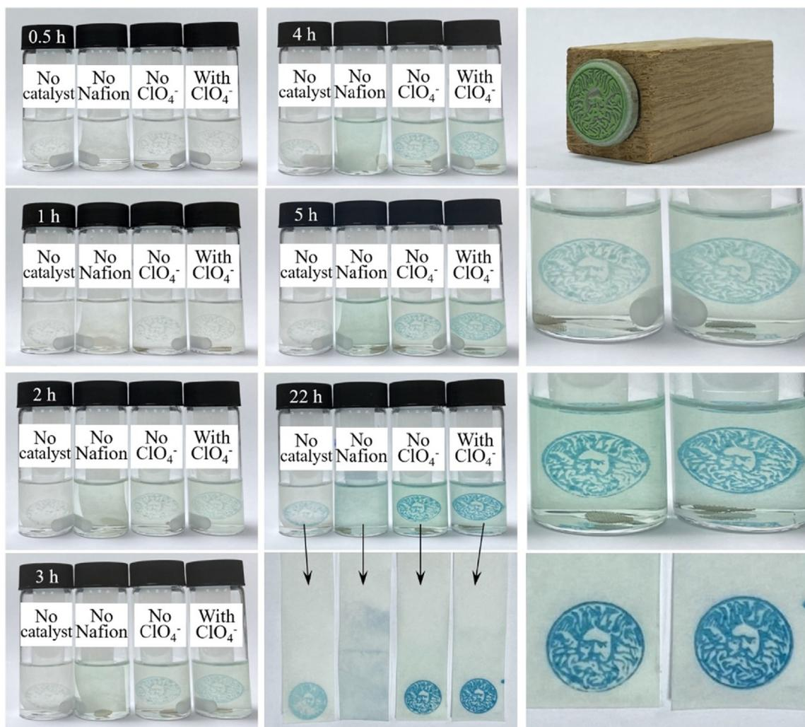
**Fig. 13.** Effects of Nafion ionomer printed on a filter paper on the TMB colour response with/without 50 mM  $\text{ClO}_4^-$  for 10 mM  $\text{HCOOH}/\text{HCOONa}$  concentration at pH 3.75. Photographs of 580  $\mu\text{M}$  TMB (A) without catalyst, (B) without Nafion, (C) in the absence of  $\text{ClO}_4^-$ , and (D) with  $\text{ClO}_4^-$  (stirred in the dark, 33 % DMSO, 11  $\text{cm}^3$ ) as a function of reaction time.
