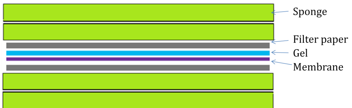
Figure 2-8 Assembly of the sponges, filter papers, nitrocellulose blotting membrane and gel for Western blotting of proteins.
