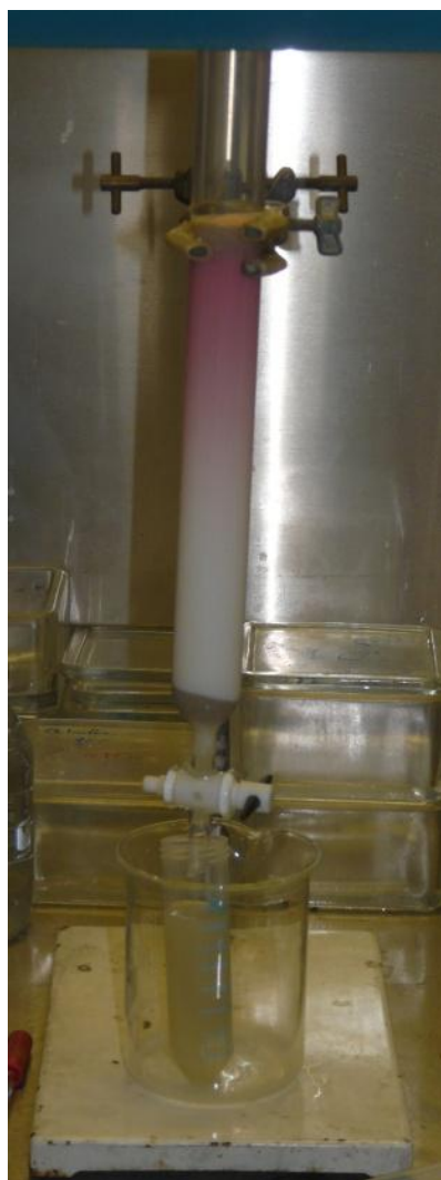
Figure 2-13 XAD-16 Column with adsorbed PRE. Using H 2 O to fraction the yellow tannin devoid solution being collected, leaving the red total pomegranate tannins (TPT) on the column.
