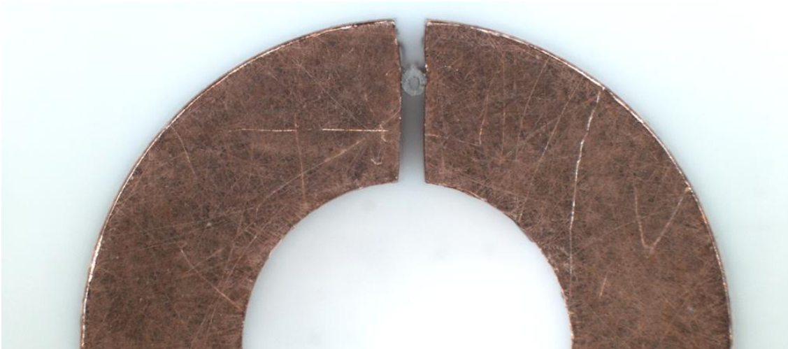
Figure 6.21: Photomicrograph of the gap section of the split ring resonator showing a cleaved section of Teflon® AF microcapillary
