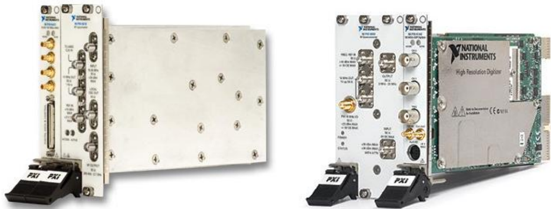
Figure 4.21: The NI PXI-5670 VSG (left) and the NI PXI-5661 VSA (right) shown withdrawn from the PXI chassis where they are normally mounted [35].
