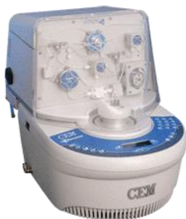
Figure 6.26: Examples of high-tech single-mode resonant cavity microwave reactors aimed at laboratory synthesis – the CEM Voyager continuous flow system (left) [30] and the Anton Paar Monowave (right) [31] – both offering fibre optic thermometry-based heating control
