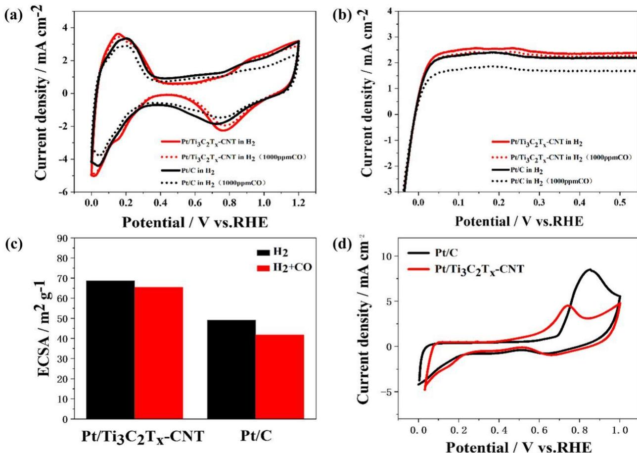
**Fig. 3** a CV curves for Pt/Ti<sub>3</sub>C<sub>2</sub>T<sub>x</sub>-CNT and Pt/C, b LSV curves for Pt/Ti<sub>3</sub>C<sub>2</sub>T<sub>x</sub>-CNT and Pt/C, c The ECSA of Pt/Ti<sub>3</sub>C<sub>2</sub>T<sub>x</sub>-CNT and Pt/C, and d CO stripping voltammograms of Pt/Ti<sub>3</sub>C<sub>2</sub>T<sub>x</sub>-CNT and Pt/C
