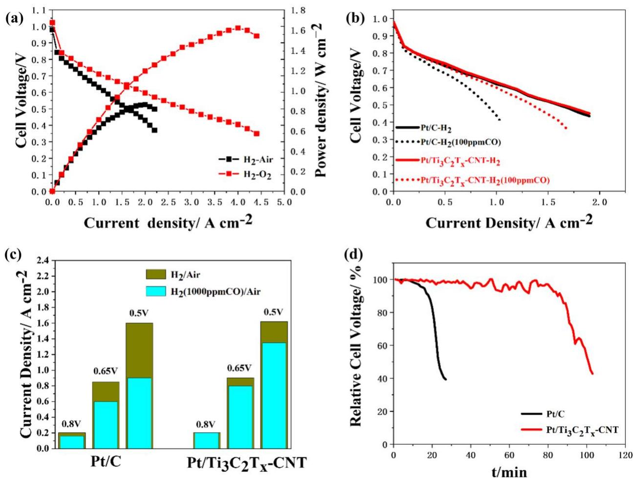
**Fig. 4** **a** Polarization curves for MEA (anode: Pt/Ti<sub>3</sub>C<sub>2</sub>T<sub>x</sub>-CNT, cathode: Pt/C), **b** polarization curves for Pt/C and Pt/Ti<sub>3</sub>C<sub>2</sub>T<sub>x</sub>-CNT as anode catalysts in the presence of 100 ppm CO under H<sub>2</sub>/O<sub>2</sub> conditions, **c** current density for Pt/C and Pt/Ti<sub>3</sub>C<sub>2</sub>T<sub>x</sub>-CNT as anode cata-
