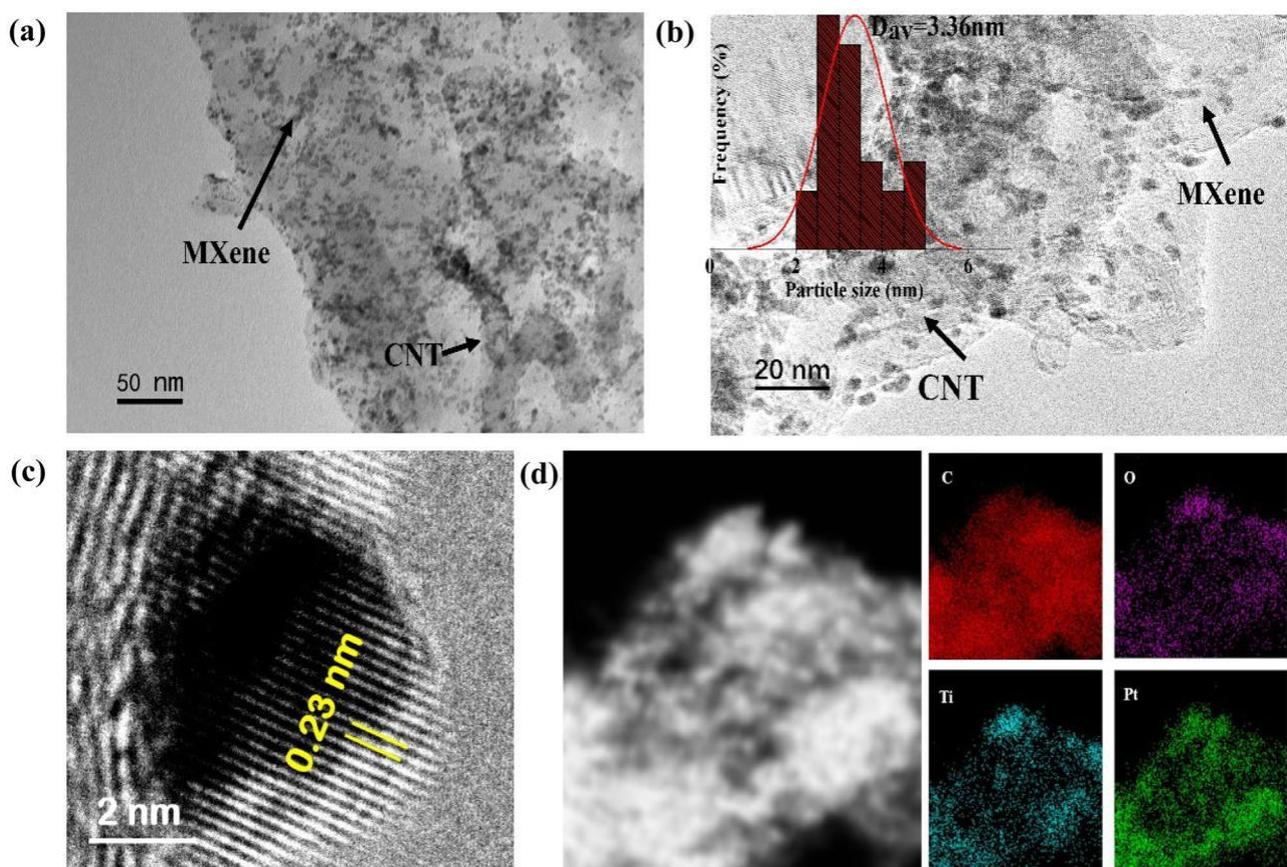
**Fig. 2** a TEM image of Pt/Ti<sub>3</sub>C<sub>2</sub>T<sub>x</sub>-CNT, b, c HRTEM image of Pt/Ti<sub>3</sub>C<sub>2</sub>T<sub>x</sub>-CNT, and d EDS mapping of Pt/Ti<sub>3</sub>C<sub>2</sub>T<sub>x</sub>-CNT
