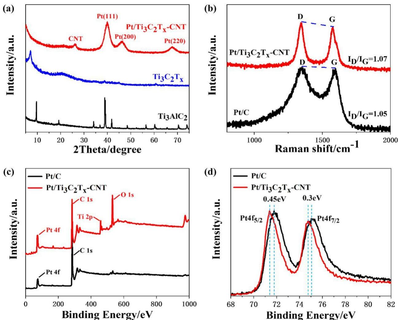
**Fig. 1** a XRD patterns of Pt/Ti<sub>3</sub>C<sub>2</sub>T<sub>x</sub>-CNT, Ti<sub>3</sub>C<sub>2</sub>T<sub>x</sub>, and Ti<sub>3</sub>AlC<sub>2</sub>; b Raman spectra of and Pt/C; c XPS spectra of Pt/Ti<sub>3</sub>C<sub>2</sub>T<sub>x</sub>-CNT and Pt/C; and d Pt 4f regions of Pt/C and Pt 4f regions of Pt/C and Pt/Ti<sub>3</sub>C<sub>2</sub>T<sub>x</sub>-CNT
