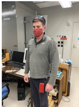
Figure 5.9 Example of measuring occupant-level exposure using a wearable dosimeter (see red device worn by the occupant on their belt).
