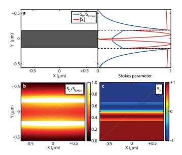
(a) Left: Schematic of dielectric structure. Right: Line plot of the stokes parameters  $S_0$  and  $S_3$  through the cross section of the waveguide. Color plot of the Stokes parameters (b)  $S_0$  and (c)  $S_3$ .
