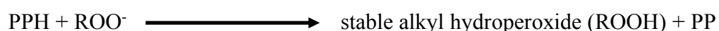
Figure 44 The Formation of stable alkyl hydroperoxide through a donation of electron by phenolic antioxidant natural product
