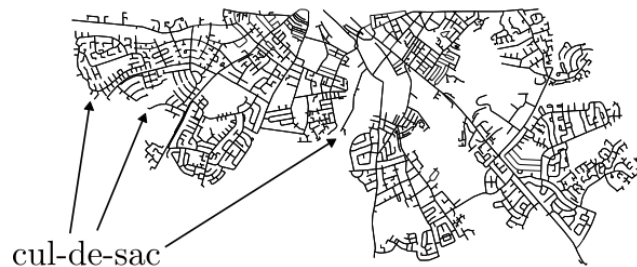
Figure 2: The street network for the city of Carlisle is displayed. This street network has the highest global entropy value of all city street networks considered. This can in part be attributed to a significant number of cul-de-sacs adjacent to important transportation corridors. A number of these are highlighted in the figure. Cul-de-sacs frequently do not belong to shortest routes and, in turn, contribute to higher entropy.
