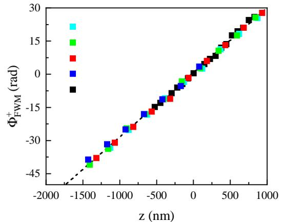
**Fig. S1 FWM phase versus NP axial position.** Phase  $\Phi_{\text{FWM}}^+$  of the co-circularly polarised FWM field measured on a set of individual 10 nm radius AuNPs while scanning their axial position using the sample nano-positioning stage. The phase has been unwrapped by multiples of  $2\pi$ , and shows a linear dependence on the axial position, as indicated.
