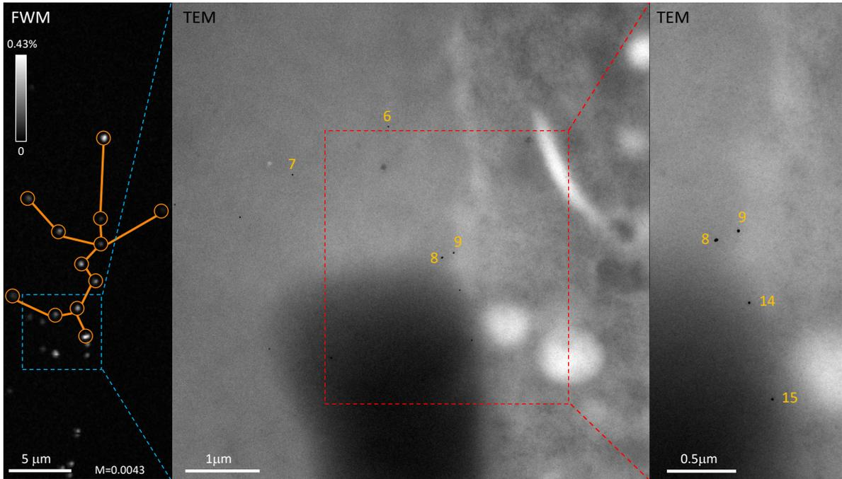
**Fig. S2 Additional 10nm radius AuNPs for shape analysis.** Overview TEM compared with the FWM imaging in Fig. 1c showing additional AuNPs, numbered as 14 and 15, below those indicated as number 8 and 9. For AuNP 15 a high magnification TEM was acquired and was included in the shape analysis in Fig. 2.
