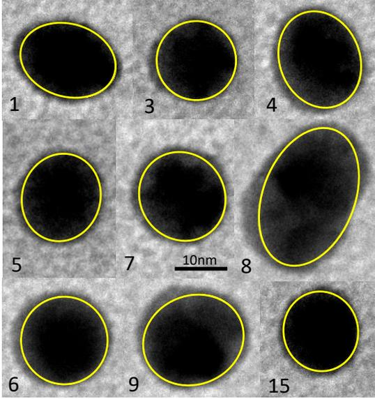
**Fig. S3 Fits of ellipse shape on TEM.** High-magnification TEM images of selected nanoparticles (numbered as in Fig. 1c with the addition of AuNP 15) fitted with an ellipse shape (shown in yellow) using a threshold such that the area of the fitted ellipse is 80% of the area shown in Fig. 2.
