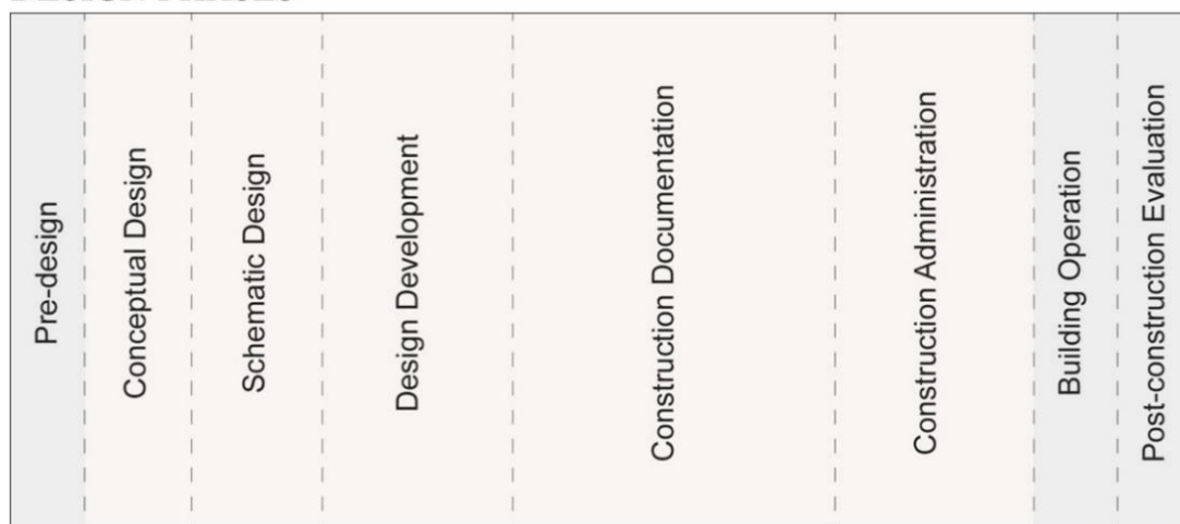
Figure 3.1: Typical architectural design phases.
