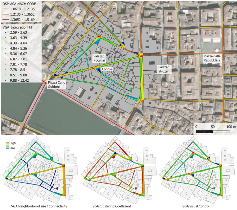
Fig. 3 Normalised Angular Choice core (15% highest NACH R_n values) in OSMnx ‘Firenze walk’ network and VGA Integration, Connectivity, Clustering and Control indices in the ‘Rucellai trade’ district. The colour-coded maps show Palazzo Rucellai’s central location between a former junction for the wool production (Piazza Carlo Goldoni) and the old market (Piazza della Repubblica) and its neighbourhood-level hierarchies. Image: C. Pezzica 2023
