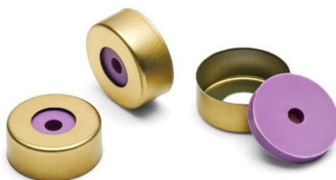
Figure 4.14: Custom clamped brass caps with the purple septum which the HiSorb penetrates prior to extraction.
