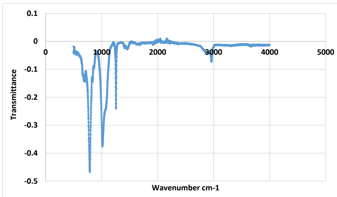
Figure 4.10: Graphical demonstration of FTIR data for PDMS crosslinked with N,N-Bis[3-(methylamino)propyl]methyleamine.
