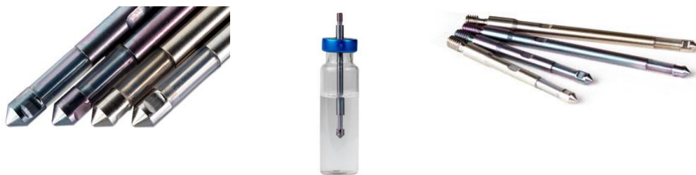
Figure 1.8: HiSorb probes and immersive sampling of organic compounds [79].
