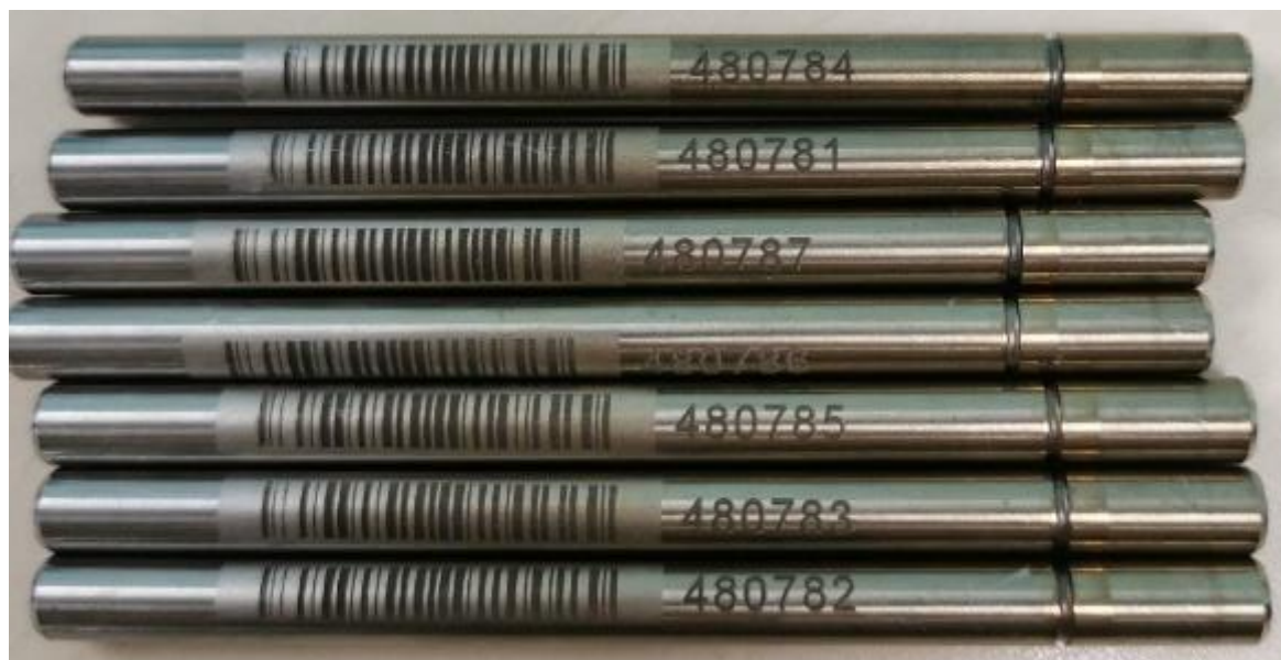
Figure 2.2: Stainless steel Tenax TA thermal desorption tubes used for spiking with calibration standards ranging from 250 - 1 µg/mL.
