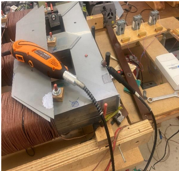
Figure 3- 20: Rotary Tool for laminations insulation removal
