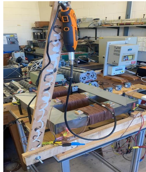
Figure 3- 20: Rotary Tool for laminations insulation removal
