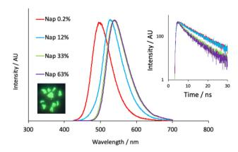
Fig. 4 Solid state emission spectra of Nap-PA-CHO ( $\lambda_{\rm ex}=410$  nm) at different dopant levels. Inset: the corresponding decay profiles ( $\lambda_{\rm ex}=295$  nm) for the different materials (fits yielding lifetimes of 8.0, 7.9, 6.8 (80% weighting) and 2.6% (20% weighting), 7.3 (71% weighting) and 2.4 ns (29% weighting) for Nap dopant levels of 0.2%, 12%, 33% and 63%, respectively).
