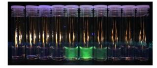
Fig. 3 Eluted GPC solvent showing the emission from the yellow (green-emissive) Nap-PA-CHO polymer in vials 5-7 ( $t_R = 14-17$  min; each vial = 1 min i.e. 1 ml.)
