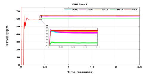
Figure 8. PV output power under PSC case 2.
