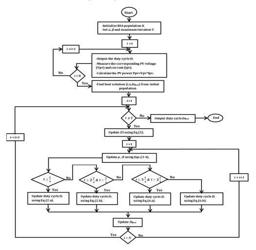
Figure 3. RSA-MPPT based flowchart.
