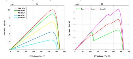
Figure 2. PV characteristic curves (a) under uniform solar irradiance and (b) under PSC.
