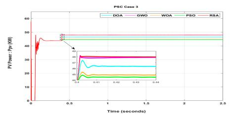
Figure 9. PV output power under PSC case 3.
