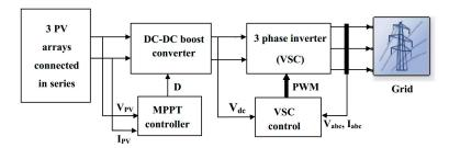
Figure 1. Block diagram of the grid connected PV system.
