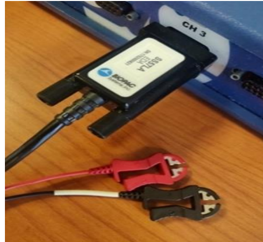
Figure 8.2.3 – SS57LA EDA lead. connects to a single input channel (e.g., CH3) to record EDA.
