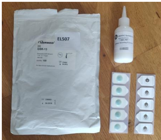
Figure 8.2.4 – Disposable EL507 electrodes and GEL101A isotonic electrode gel. Latex-free electrodes, Ag/AgCl contact, wet gel (0.5% chloride salt), electrode contact diameter: 11 mm, electrode contact area: 95 mm 2 , size: 27 mm x 36 mm, backing: 1.5 mm thick foam.
