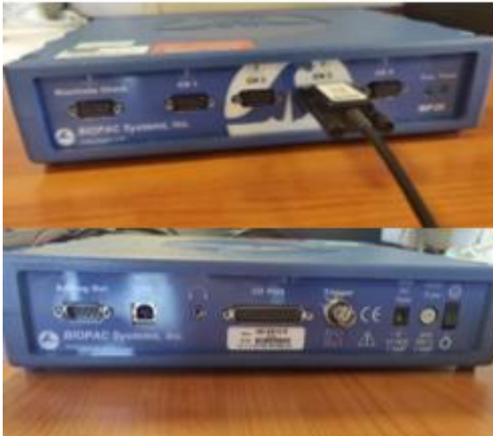
Figure 8.2.2 – BIOPAC MP36 data acquisition unit features. Four channels (CH1-4), “electrode check” for electrode impedance, direct current (DC) input (12 VDC at 1 Amp), USB 2.0).
