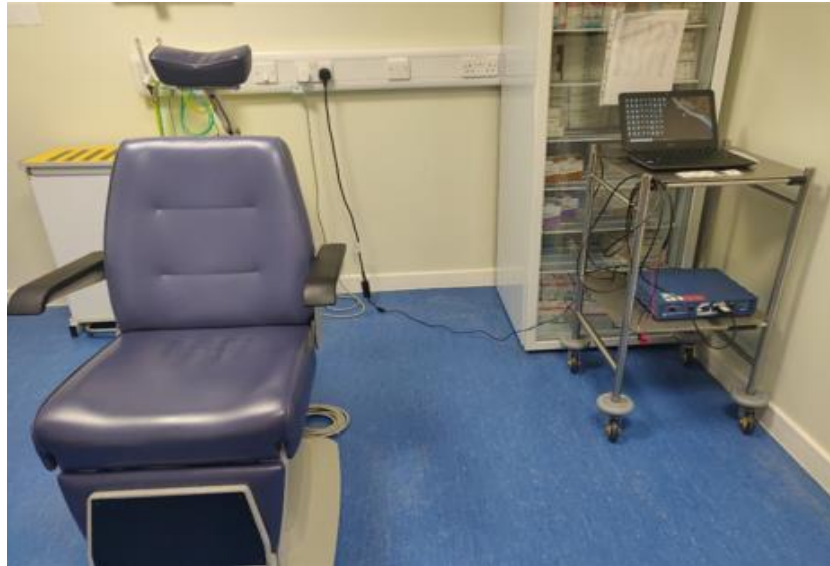
Figure 8.2.6 – Experiment set-up at the hospital site (injection room). The injection is performed while the patient is sitting on a reclining chair. BIOPAC MP36 data acquisition unit connected to notebook laptop ( Acer TravelMate B117-M ) for data recording.
