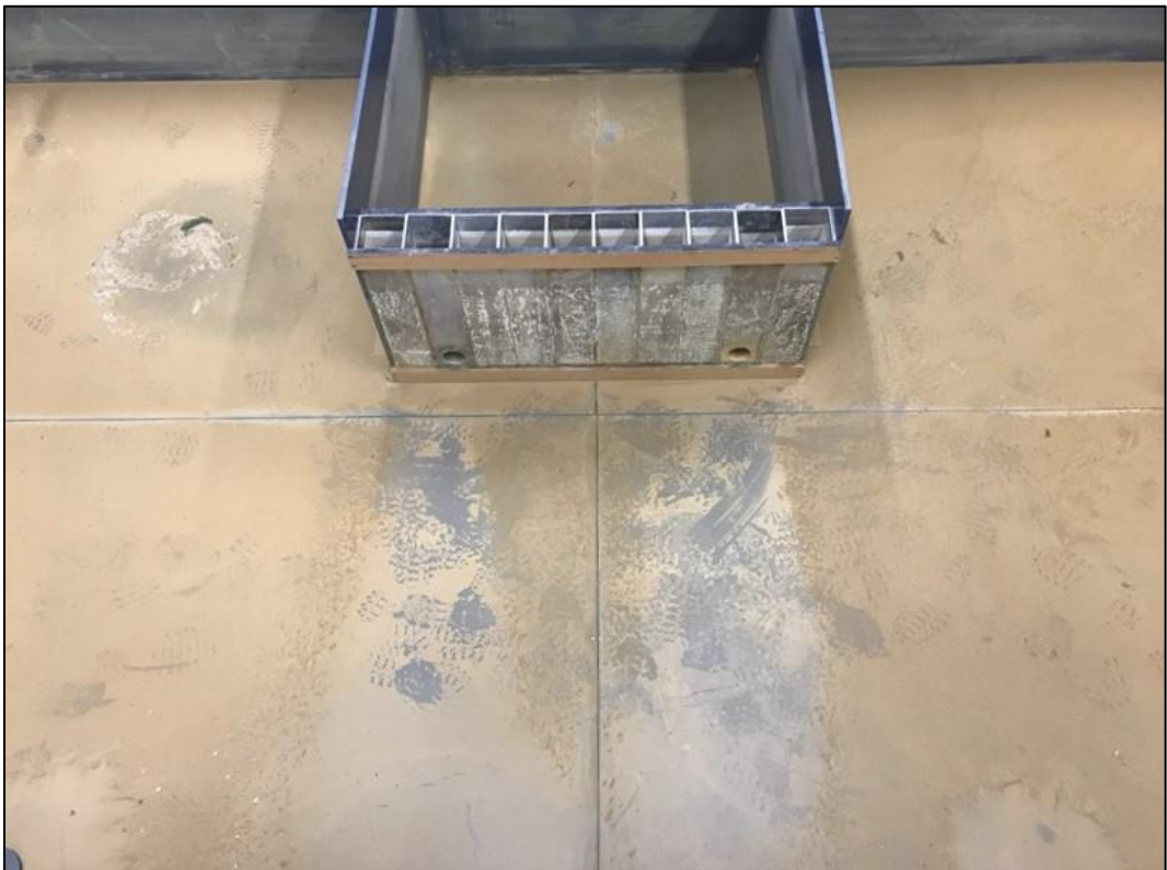
Figure 4.88 Evidence of whirlpool left in dust once tank is emptied.
