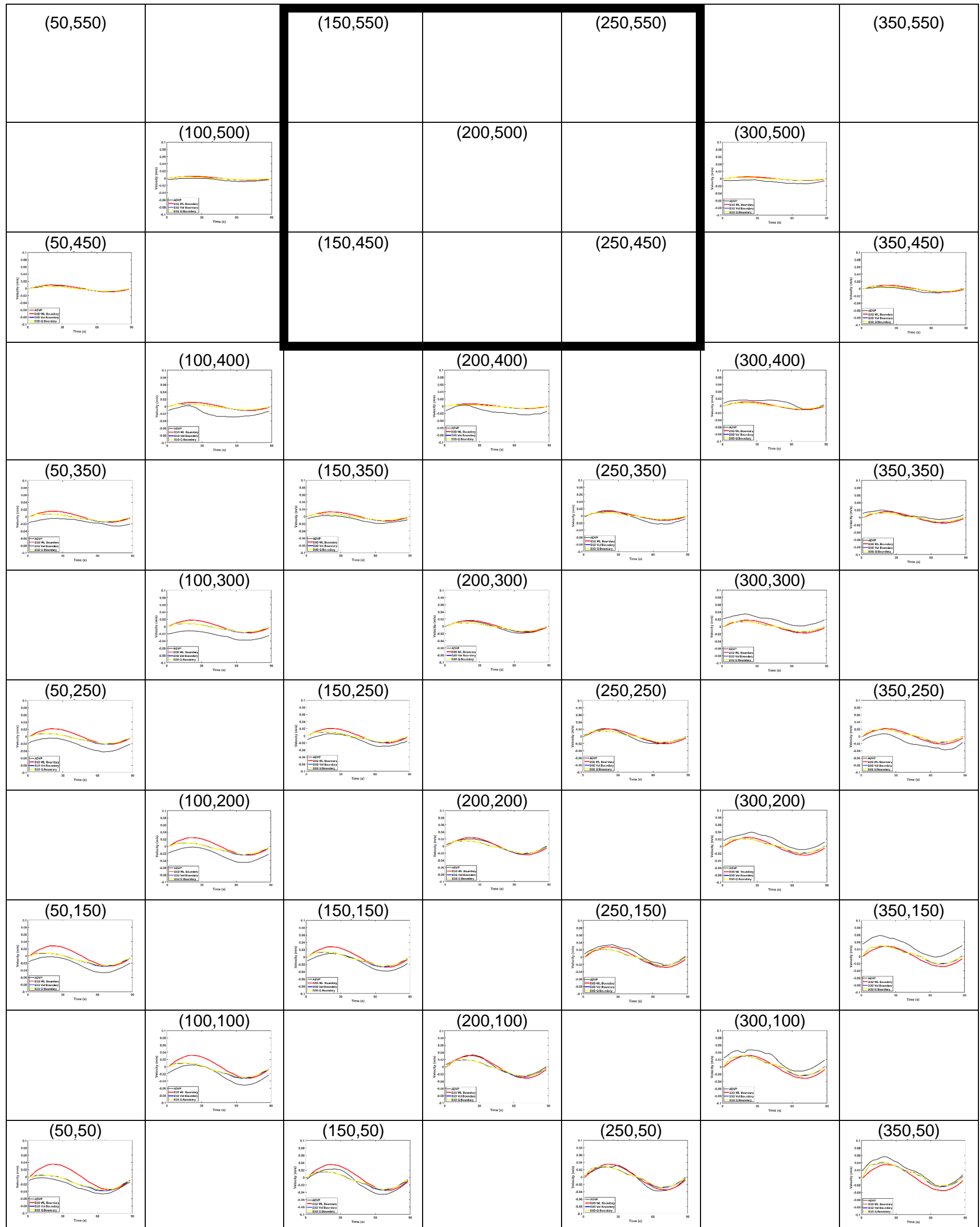
Figure 7.5 Experiment S0 depth averaged velocity results for different inflow boundaries in Delft3D, black: ADVP measurements, red: water level inflow boundary, blue: velocity inflow boundary, yellow: discharge inflow boundary results.
