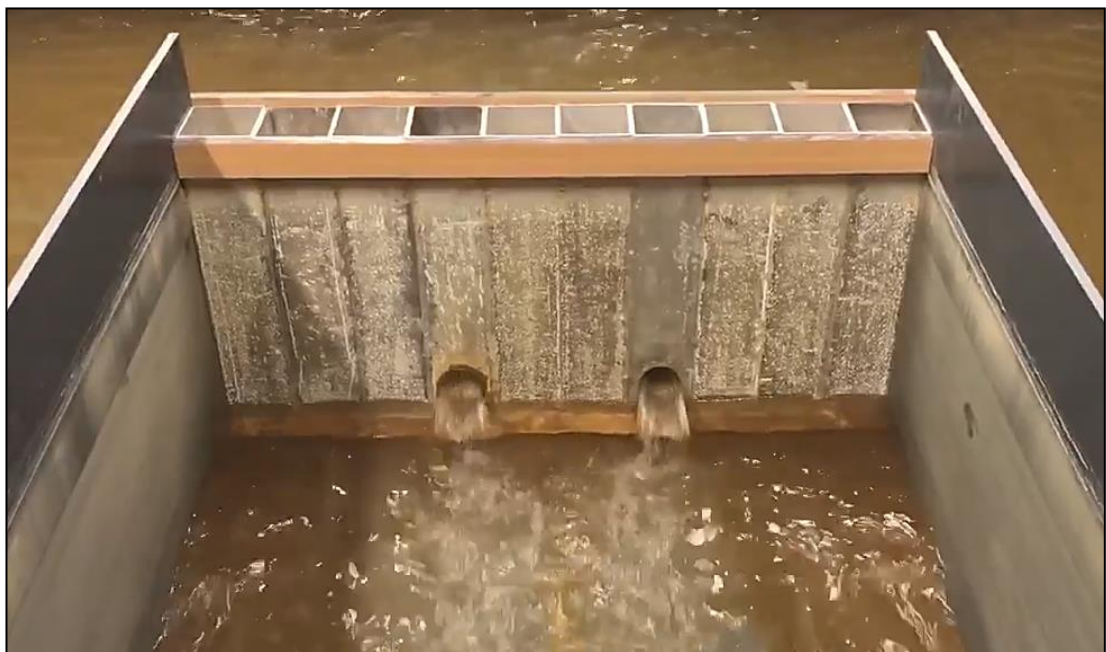
Figure 3.7 Example of box section arrangement with two turbine opening box sections and eight blank box sections.
