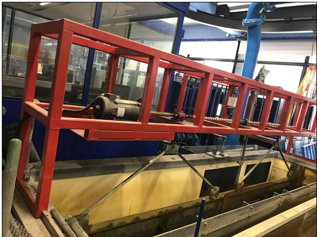
Figure 3.3 Photograph of tidal basin weir gate.
